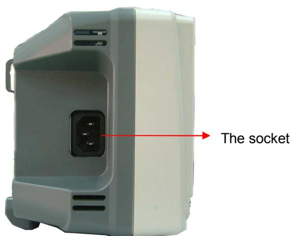
Figure 2-1 Connect power line
