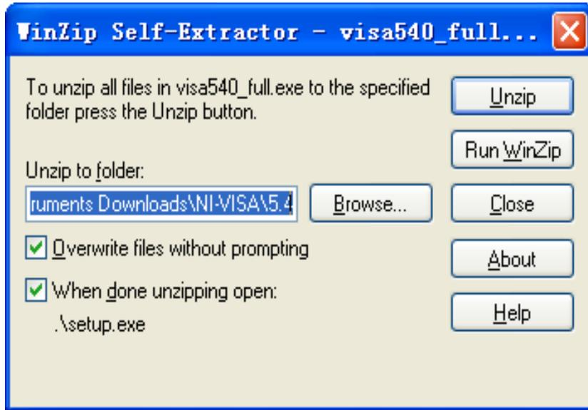
b. Click Unzip, the installation process will automatically launch after unzipping files. If your computer needs to install .NET Framework 4, it may auto start.
