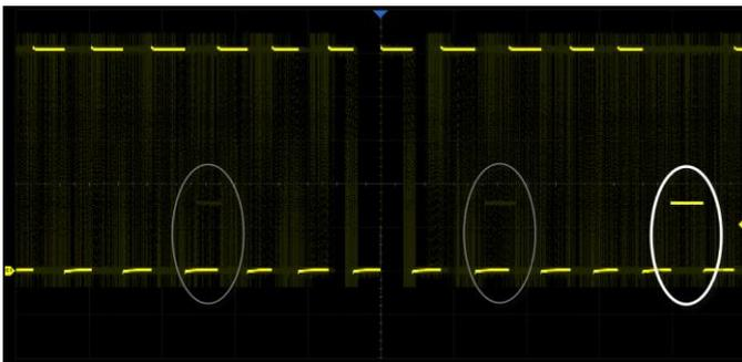
With a waveform update rate of up to 170,000 wfms/s, the oscilloscope can easily capture unusual or low-probability events. In Sequence mode, the waveform capture rate can reach 750,000 wfms/s
