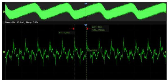
Using hardware-based Zoom technique and record length of up to 500 Mpts, users can select a slower timebase without compromising the sample rate, and then quickly zoom in to focus on the area of interest
