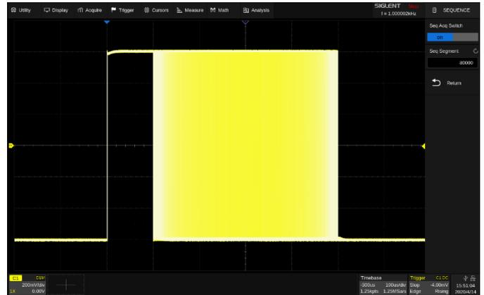
Segmented memory collection will store the waveform into multiple memory segments (up to 80,000) and each segment will store a triggered waveform as well the dead time information. The interval between segments can be as small as 1.3 μs. All of the segments can be played back using the History function
