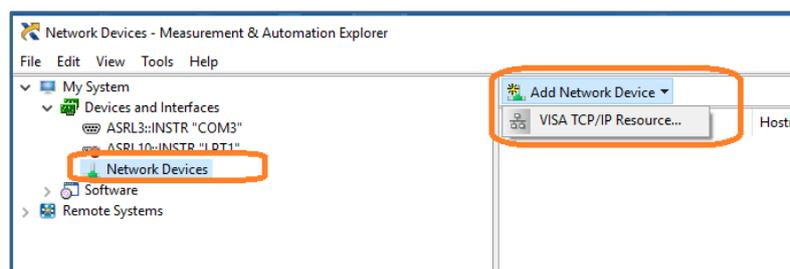
3. Select Manual Entry of LAN instrument, select next, and enter the IP address as
