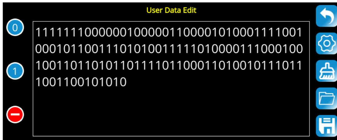
You can input 0|1 in the input box manually or insert PN7|PN9|PN15 data bits by pressing
