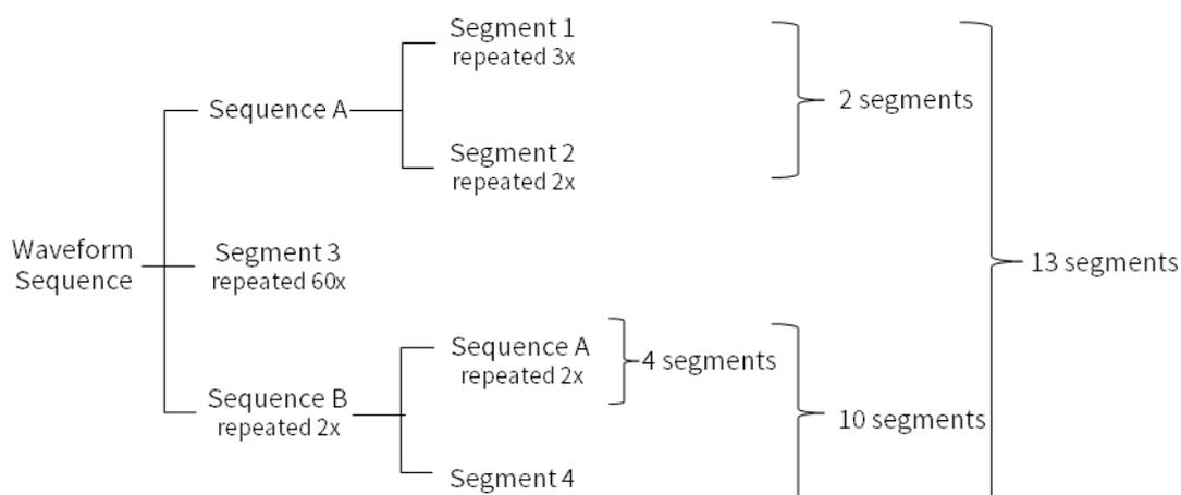
For example, if a waveform sequence contains 24 segments and one nested sequence with 10 segments, the nested sequence can only repeat  $(1024-24) / 10 = 100$  times at most.
