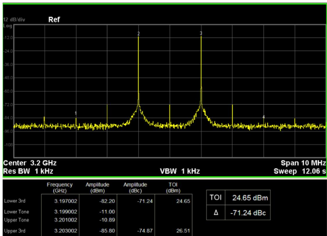
**Note:** IQ compensation can be performed through **I/Q Control**->**I/Q Adjustment** menu of the SSG. For example, when the IQ modulation signal shows a significant local oscillator leakage, it can be solved by alternately adjusting the Offset of I and Q.
