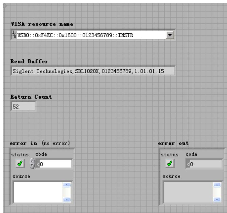
In this example, the VI opens a VISA session to a USBTMC device, writes a command to the device, and reads back the response. In this example, the specific command being sent is the device ID query. Check with your device manufacturer for the device command set. After all communication is complete, the VI closes the VISA session.
