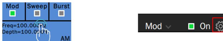
Clicking in the Mod, Sweep or Burst switch area of the Modulation/Sweep/Burst setting block allows you to quickly turn the corresponding function on/off.
