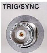
The TRIG/SYNC port on the rear panel is automatically set as the trig input/output function when the frequency sweep or burst is turned on. In other cases, it is the sync output function by default.
