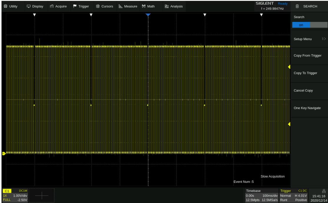
Turn on the Zoom function to observe the full view of the frame and the detail of the third dwarf pulse at the same time:
