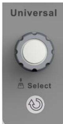
When the parameter setting area is highlighted, the Universal Knob can be used to adjust the parameter. Press the knob to select an option from the list. The default function of the Universal Knob is to adjust the intensity of the waveform traces.
