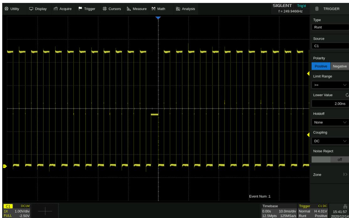
Then turn on the Search function and operate *Copy from Trigger* in the search dialog box so that the oscilloscope searches for the dwarf pulses according to the same setting as the trigger.
