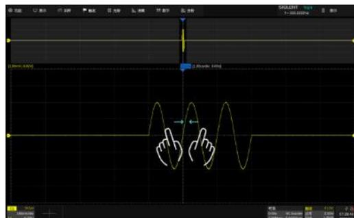
Adjust the horizontal scale of Zoom window by horizontal pinch and spread in the zoom area of the main window or the Zoom window
