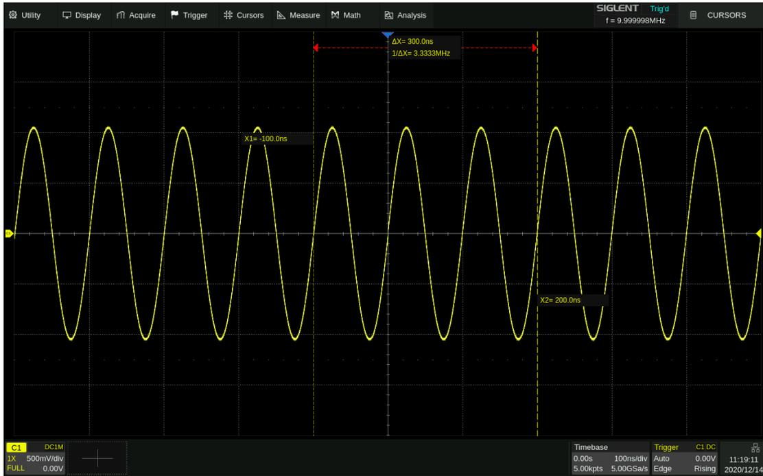
Fixed position, timebase is changed to 100 ns/div, the grid number of X cursors (-1div, 2div) remains fixed. The value of X1 and X2 is changed to -100 ns, 200 ns.
