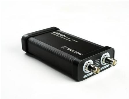
The SAG1021I function/arbitrary wave generator module is capable of generating variant waveforms with frequencies up to 25 MHz and amplitudes up to  $\pm 3$  V. Its output terminals are isolated from the ground of the oscilloscope.
