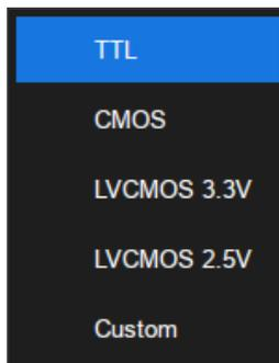
The configurable logical level includes TTL, CMOS, LVC MOS 3.3 V, LVC MOS 2.5 V, and Custom.
