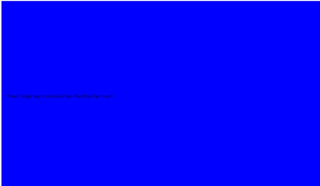
Press the "Single" button to switch to red and green display mode. Observe whether there is any color distortion, bad pixel, or scratches on the screen. Press the "Run/Stop" button to exit the screen test mode.
