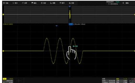
Adjust the horizontal position of the zoom area by dragging left and right in the zoom area of the main window or waveform in the Zoom window
