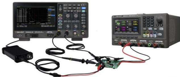
SDS800X HD can control the USB AWG module or control an independent SIGLENT SDG instrument, scan a device's amplitude and phase frequency response, and display the data as a Bode Plot. There is also a Vari-level Mode for accurately measuring Power Supply Control Loop Response (PSRR).
