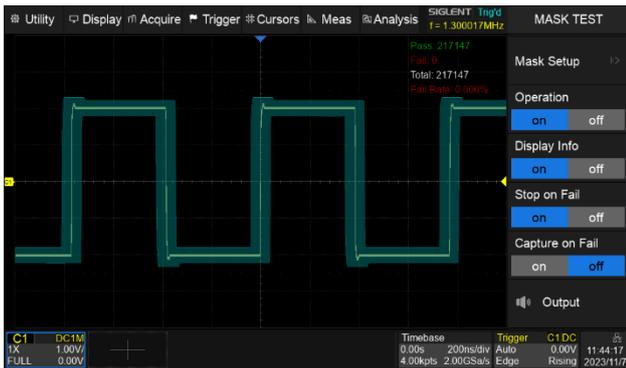
The oscilloscope utilizes a hardware-based Mask Test function, performing up to 80,000 Pass / Fail decisions each second. It is easy to generate user-defined test templates to provide trace mask comparisons, making it suitable for long-term signal monitoring or automated production line testing.
