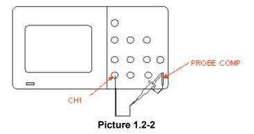
3. Press "AUTO" to show the 1 KHz frequency and about 3V peak-peak square wave in couple seconds
