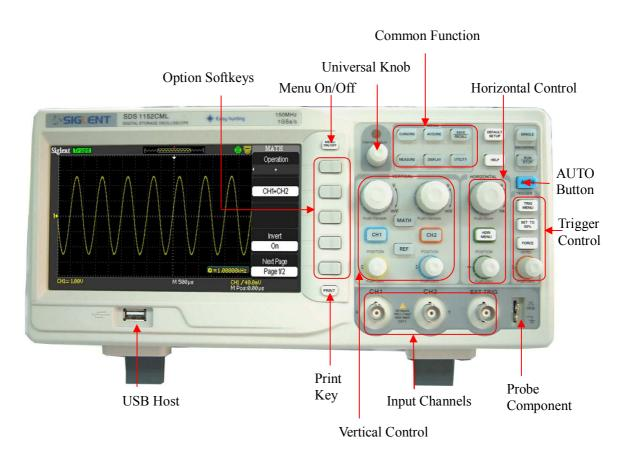
Picture 1.1-1 SDS1000L Series Front Panel
