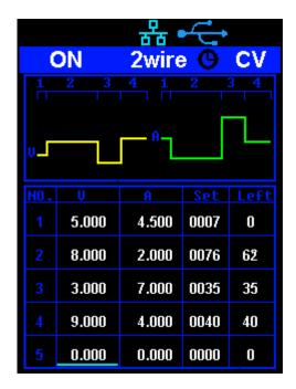
After starting the timer function, the timer will stop if you press the On/Off button to switch off the channel output. When the channel output is turned on again, the timer will continue counting from the last point in time it stopped. After the countdown steps have completed the timer will turn off automatically.
