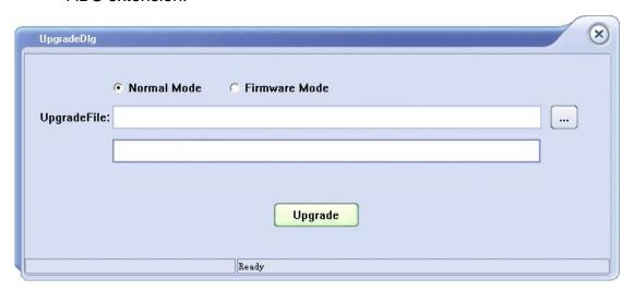
4. As is shown in figure 4, click Upgrade button to begin the upgrade. The upgrade is finished when the progress bar completes and the instrument will automatically run the version after the upgrade.
