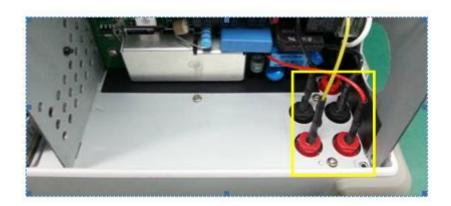
9. Remove the cable and unscrew all the screws,then you can remove the PCBA.
