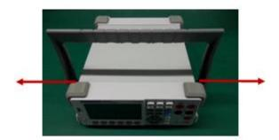
3. Unscrew the two captive screws in the rear bezel and remove the rear bezel as indicated by the arrow shown below
