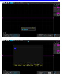
• For SDS1000X-E series, the following command saves the current setup to root directory of the USB memory device in a file called "TEST.xml". Then you can see the file on PC.
