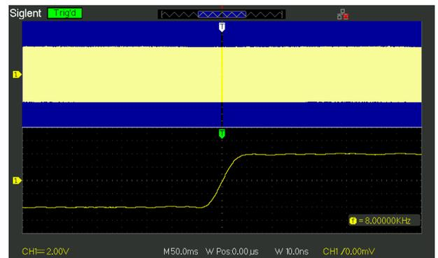
Zoom can extend a partial segment of the waveform, giving the user not only an overview of the whole signal but also a detailed view of the zoomed-in segment. The Zoom feature is a convenient way to locate a specific segment of a signal while zooming in to see the details.
