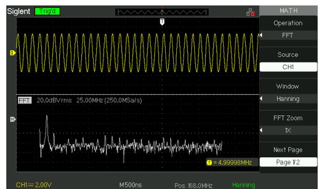
SDS1000DL+/CML+ provides 5 kinds of math operation: +, -, \*, /, FFT, supporting channel waveform and FFT waveform in either split display windows or both signals appearing on the full screen.
