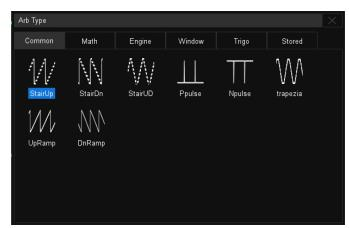
The built-in waveform generator can output waveforms with up to 50 MHz frequency and  $\pm 3$  V amplitude. Six basic waveforms together with multiple types of predefined waveforms and as user defined arbitrary waveforms are supported.
