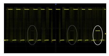
With a waveform update rate of up to 120,000 wfm/s, the oscilloscope can easily capture low-probability events. In Sequence mode the waveform capture rate can reach 500,000 wfm/s.
