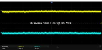
500 MHz bandwidth (at 2 GSa/s sample rate with 500 MHz Low noise floor: Only 80 μV rms at 500 MHz bandwidth. bandwidth option).
