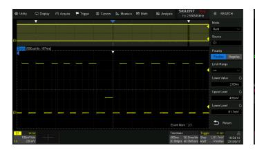
The SDS2000X Plus can find events within a record and history based on user specified trigger conditions. Navigate browses through Events flagged by the Search, plays back history frames or continuously moves the delay position on long records (useful in zoom view).
