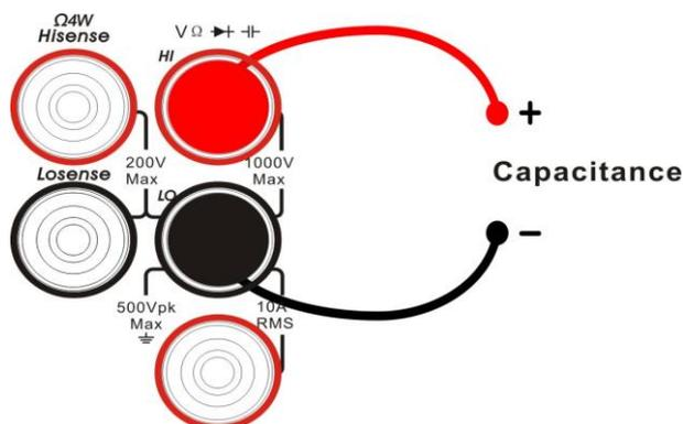
Diagram 2- 18 Sketch Map for Measuring Capacitance
