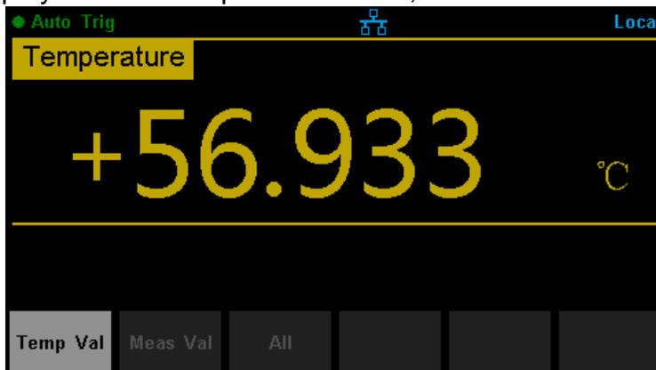
Diagram 2- 31 Choose Display Mode of Temperature Measurement
