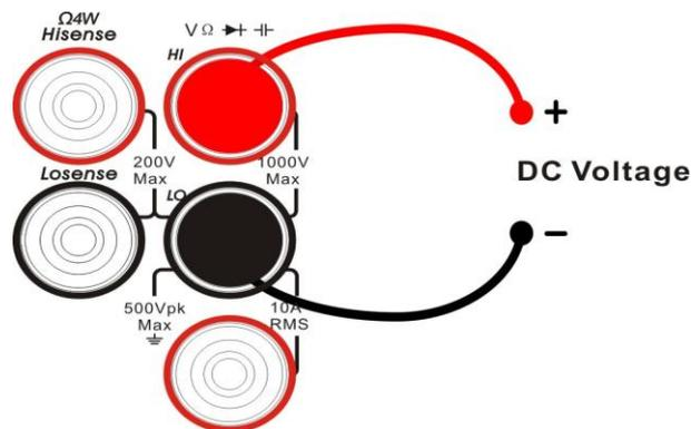
Diagram 2- 5 Sketch Map for Measuring DC Voltage
