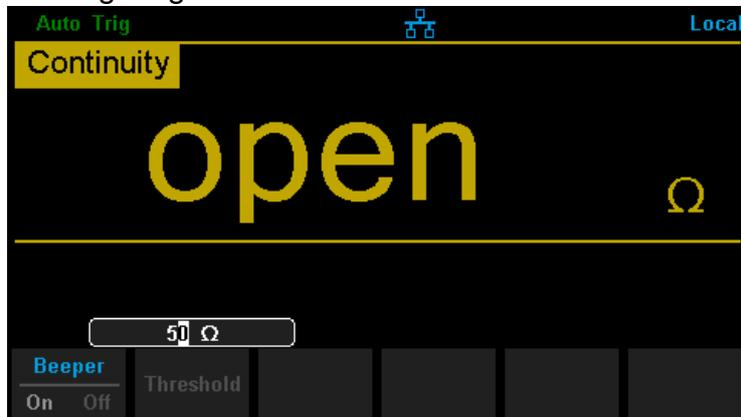
Diagram 2- 35 Set Up the Short-circuit Resistance
