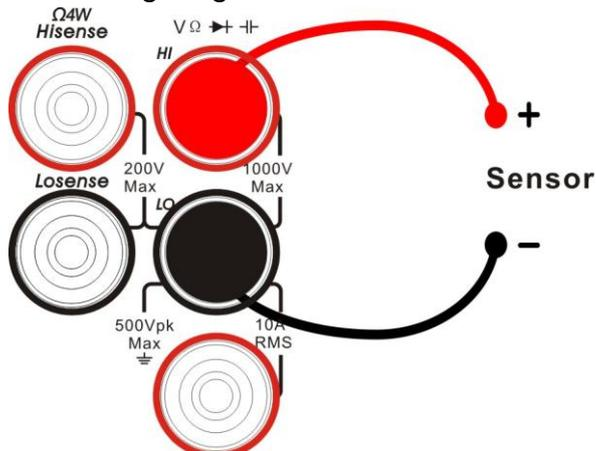
Diagram 2- 28 Sketch Map for Measuring Temperature
