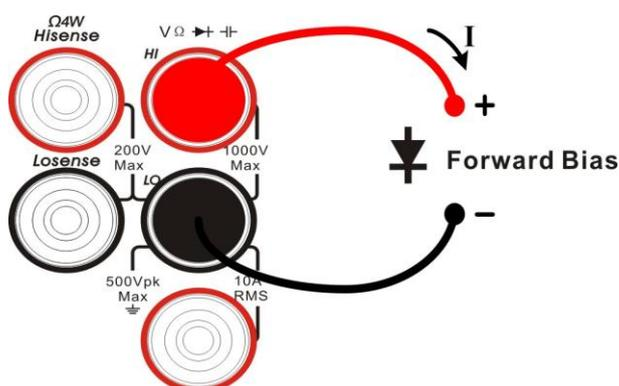
Diagram 2- 26 Sketch Map for testing Diode
