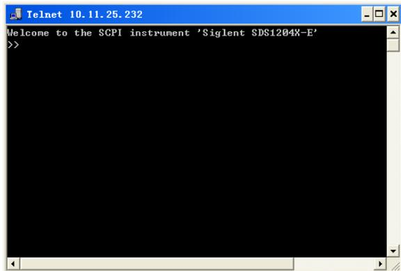
5. At the SCPI> prompt, input the SCPI commands such as *\*IDN?* to return the company name, model number, serial number, and firmware version number.
