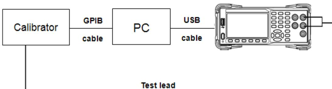
2. Verify the calibrator (Fluke 5522A) with a high precision multimeter (HP 3458A).
