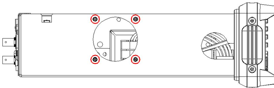
8. Remove the cable plug connected to the front panel.
