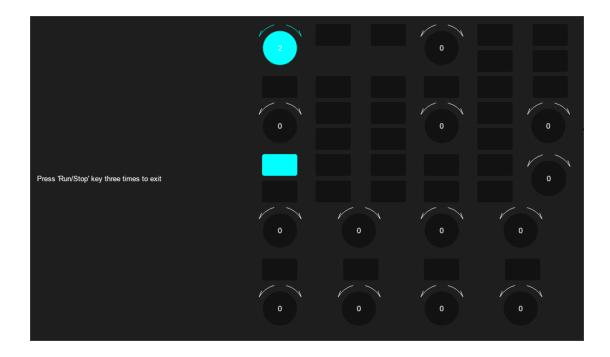
**Knob test:** Turn each knob clockwise, counter-clockwise, and press down. Observe whether the value on the corresponding knob (default 0) on the screen increases or decreases in real time and whether the knob lights up when it is pressed.
