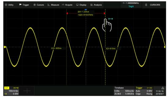
Touch the display area of  $\triangle X$  (or  $\triangle Y$ ) in M1 mode and drag it to move the two cursors simultaneously, as shown in the figure below. This is equivalent to the operation on the cursor type X1-X2 or Y1-Y2.
