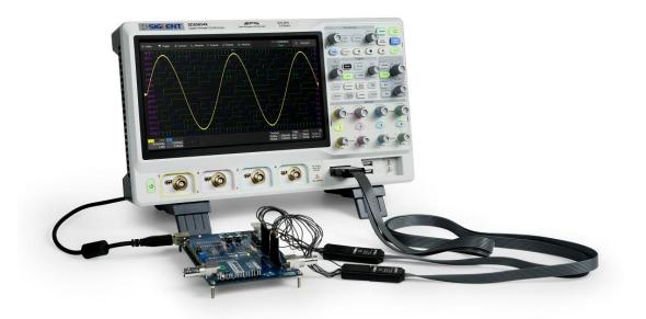
To connect the logic probe: Insert the probe, with the correct side facing up, until you hear a "click".
