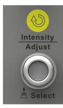
When the parameter setting area is highlighted, you can use the Universal Knob to adjustor set the parameter. Press the knob to select an option from the list. The default function of the Universal Knob is to adjust intensity of the waveform traces.
