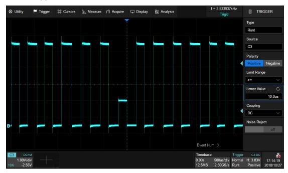
Then turn on Search function and operate *Copy from Trigger* in the search dialog box so that the oscilloscope searches for the dwarf pulses according to
