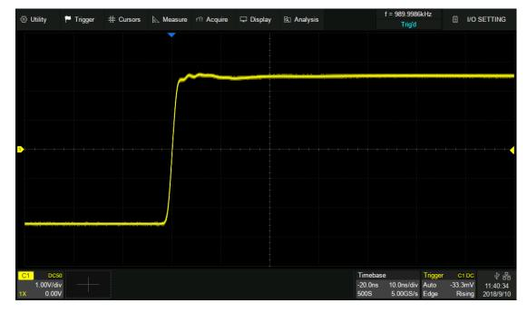
Timebase=10ns/div, Horizontal Delay=-20ns=-2div
