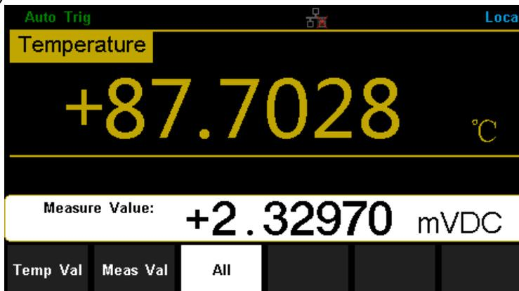
Diagram 2- 22 Choose Display Mode of Temperature Measurement
