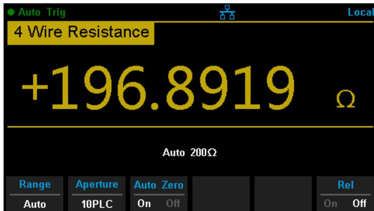
Diagram 2- 14 4 Wire Resistance Measurement Interface
