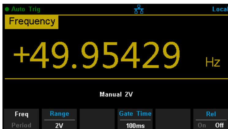
Diagram 2- 8 Set Up the Gate Time
