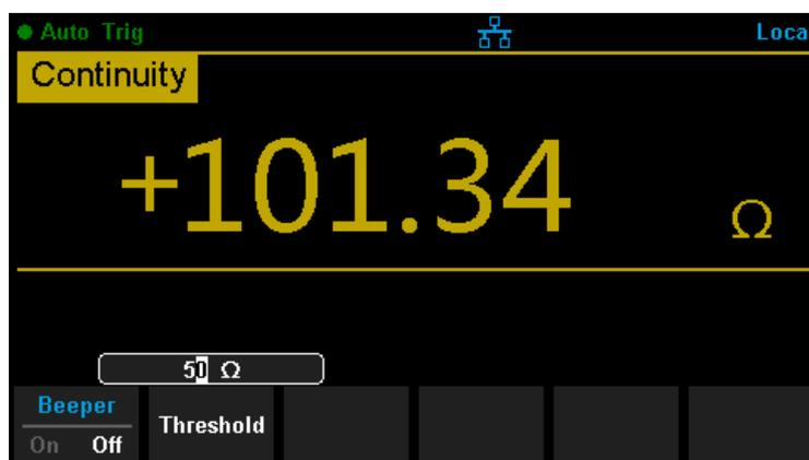
Diagram 2- 7 Set Up the Short-circuit Resistance
