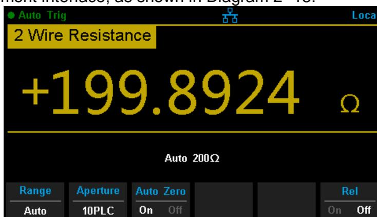
Diagram 2- 13 2 Wire Resistance Measurement Interface
