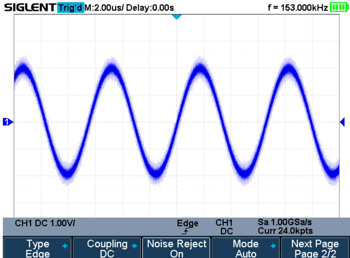
Figure 26 Turn on the Noise Reject
