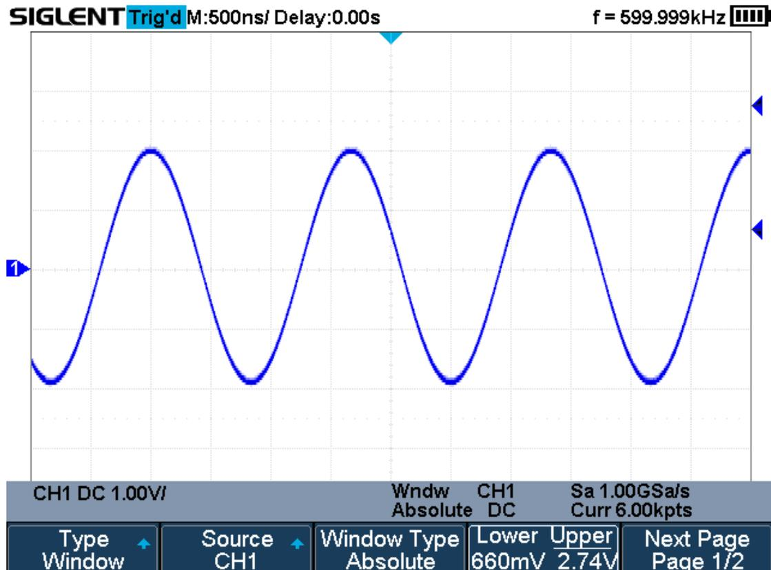
Figure 31 Absolute Window Trigger
