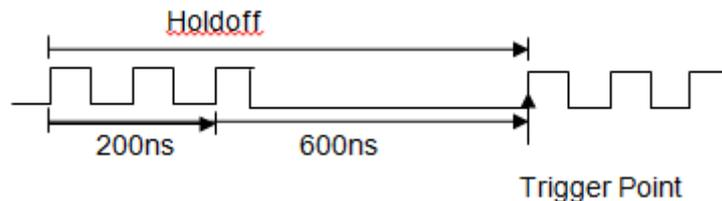
The correct holdoff setting is typically slightly less than one repetition of the waveform. Set the holdoff to this time to generate a unique trigger point for a repetitive waveform. Only edge trigger and serial trigger have holdoff option. The holdoff time of the oscilloscope is adjustable from 80ns to 1.5s.
