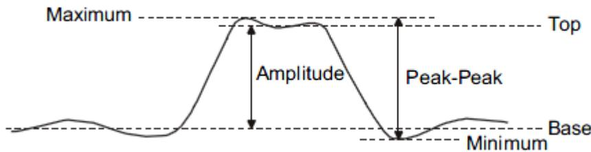
Figure 78 Voltage Measurements
