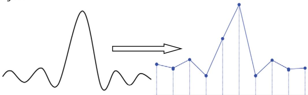
2. **Waveform Confusion:** when the sample rate is lower than twice the actual signal frequency (Nyquist Frequency), the waveform frequency reconstructed from the sample data is lower than the actual signal frequency. The most common aliasing is the jitter on fast edge.
