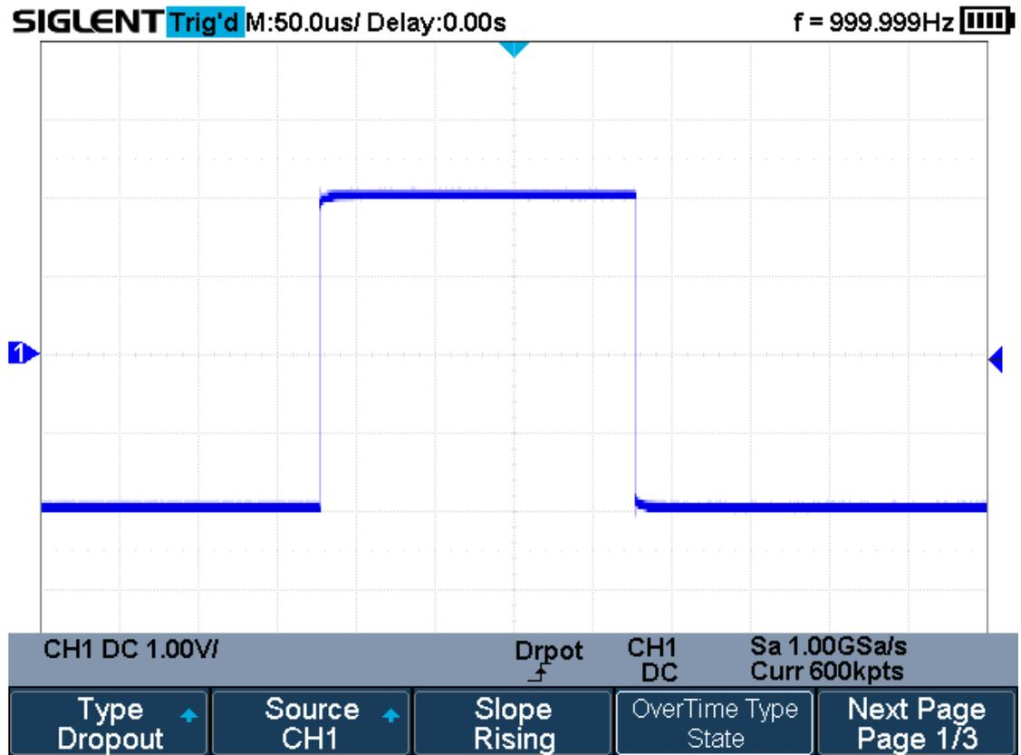
Figure 35 State Dropout Trigger
