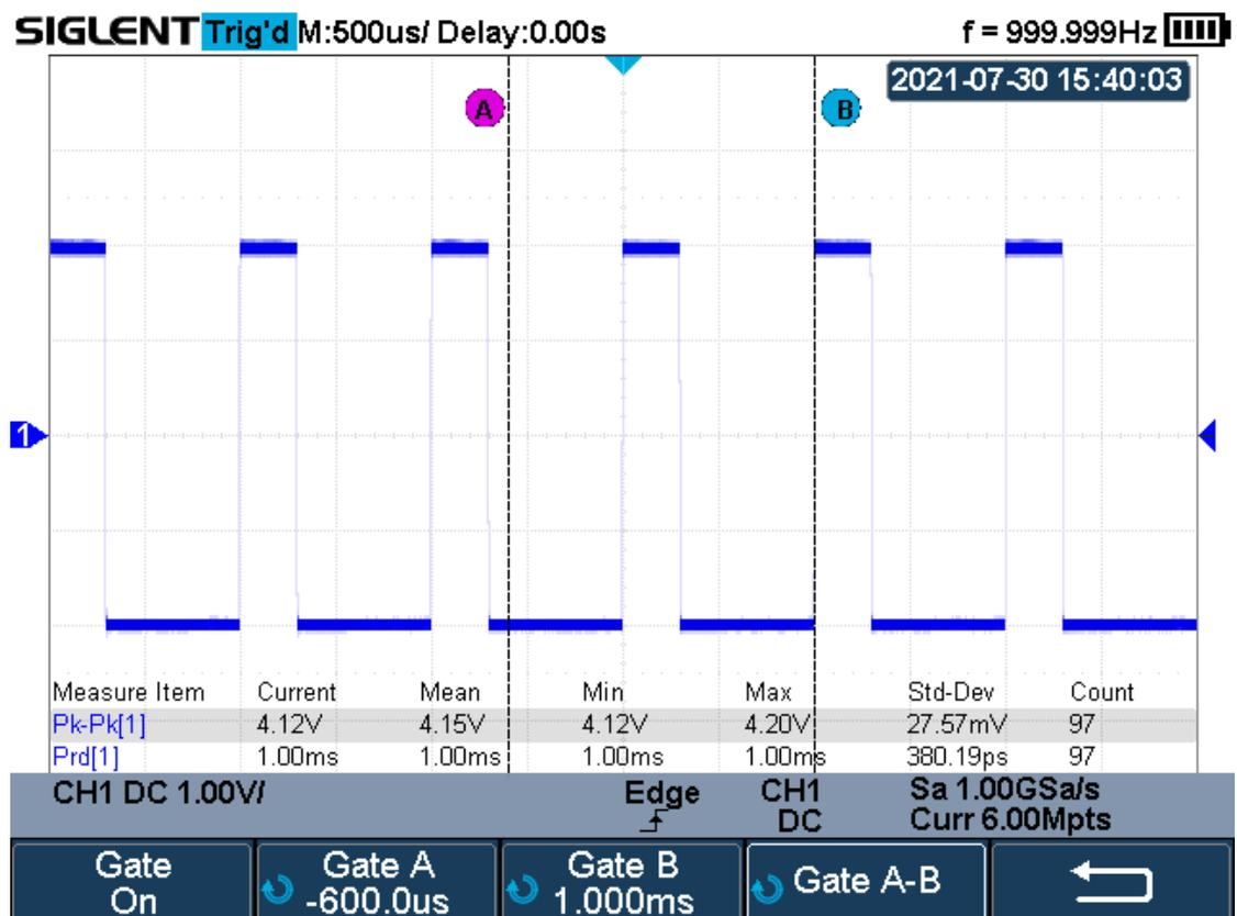
Figure 85 Gate Measurement
