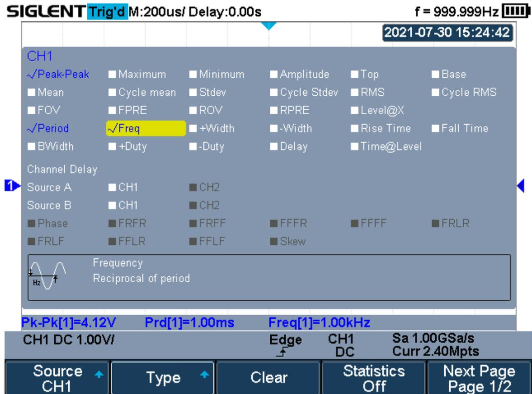
Figure 82 Select the Measurement Parameter
