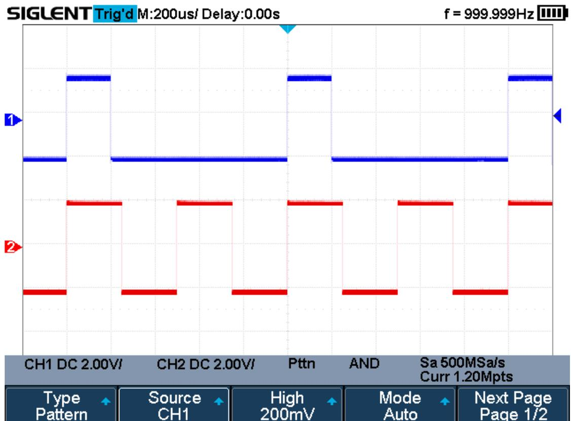
Figure 37 Pattern Trigger
