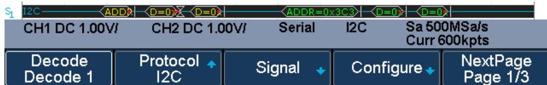
Figure 41 I2C Decode Bus Display
