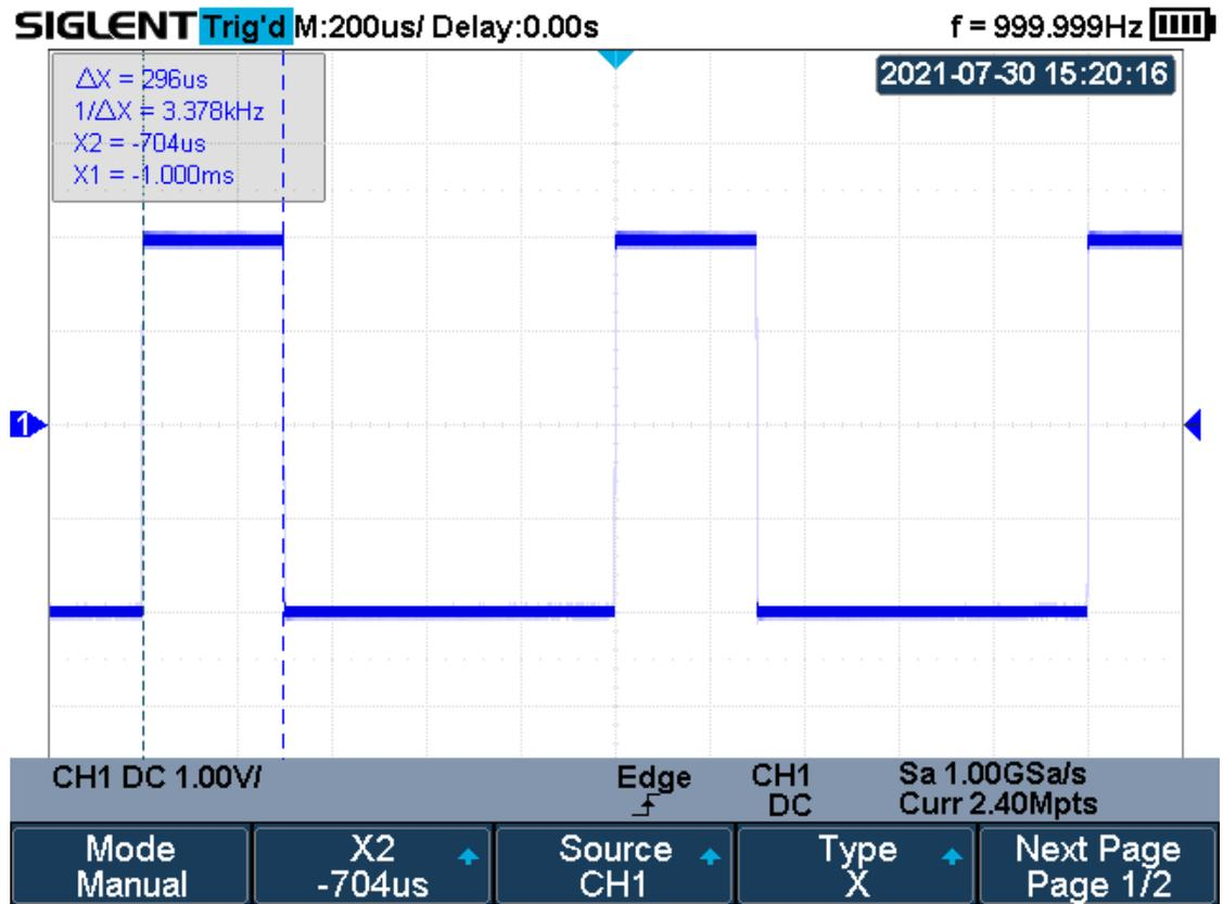
Figure 77 Measure Pulse Width
