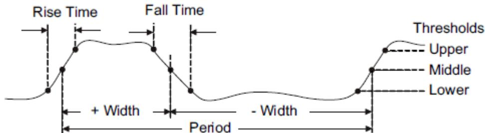
Figure 81 Time Measurements
