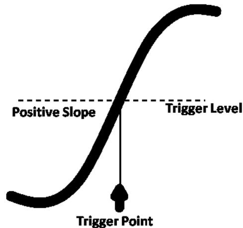
You can adjust the trigger level for a selected analog channel by pressing the **Trigger Level** button and turning the **Universal Knob**.
