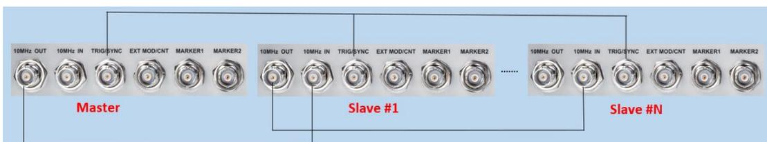
Figure 17-1 wiring diagram of multi-device synchronization
