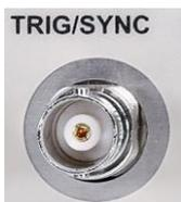
The TRIG/SYNC port on the rear panel is automatically set as the trigger input/output function when the frequency sweep or burst is turned on. In other cases, it is the sync output function by default.
