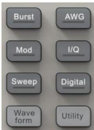
Press the **Burst** / **Mod** / **Sweep** button to quickly turn on/off the burst/modulation/sweep function and jump to the corresponding parameter setting page. When the function is turned on, the corresponding button light is on.
