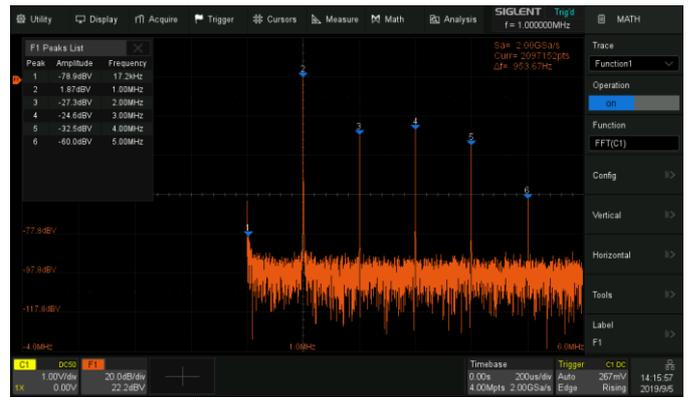
FFT supports up to 4 Mpts operation. This provides high-frequency resolution with a fast refresh rate. The FFT function also supports a variety of window functions so that it can adapt to different spectrum measurement needs. Three modes (Normal, Average, and Max hold) can satisfy different requirements for observing the power spectrum. Auto peak detection and markers are supported.
