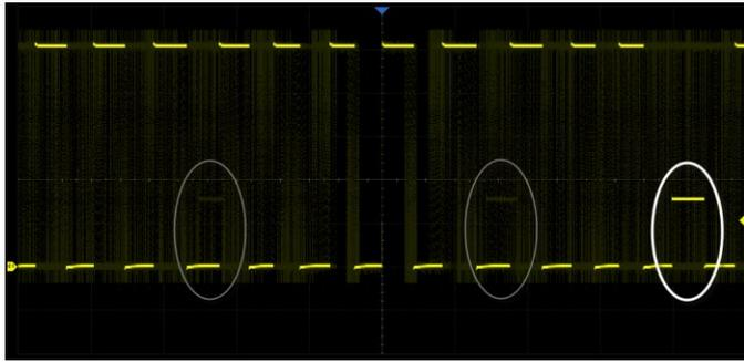
With a waveform update rate of up to 200,000 wfm/s, the oscilloscope can easily capture unusual or low-probability events. In Sequence mode, the waveform capture rate can reach 890,000 wfm/s
