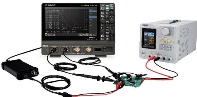
The oscilloscope can control the SIGLENT isolated USB AWG module or a stand-alone SIGLENT SDG generator, to scan the amplitude and phase-frequency response of the DUT, and display the data as a Bode Plot. This makes it possible to replace expensive network analyzers in some applications
