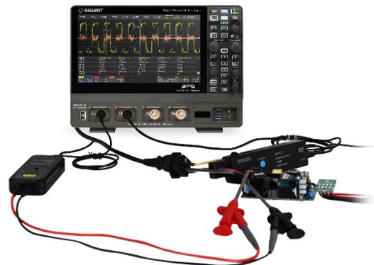
The Power Analysis option provides a full suite of power measurements and analysis, which greatly improve the measurement efficiency in switching power supplies and power devices design
