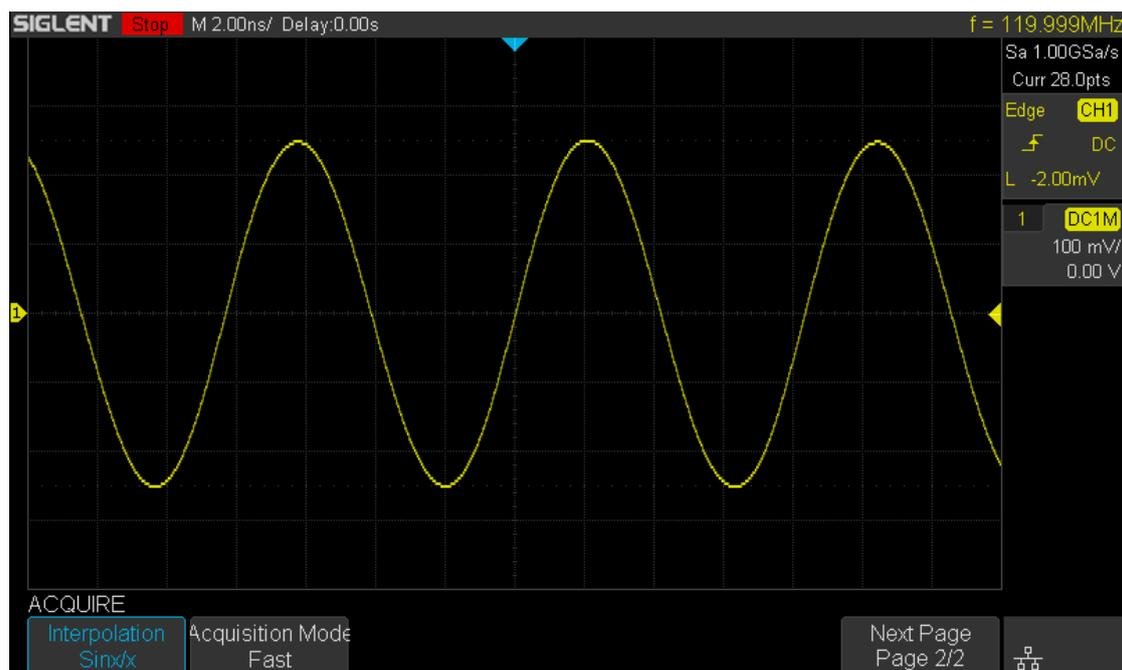
Figure 18 Sinx/x Interpolation
