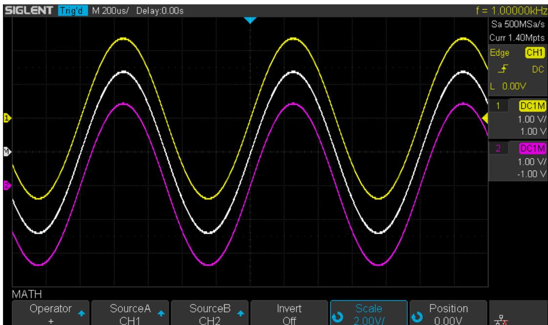
Figure 58 C1+C2 Waveform
