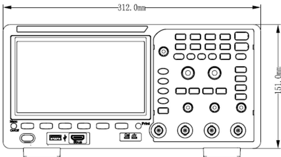
Figure 3 Front View (4-channel scope)
