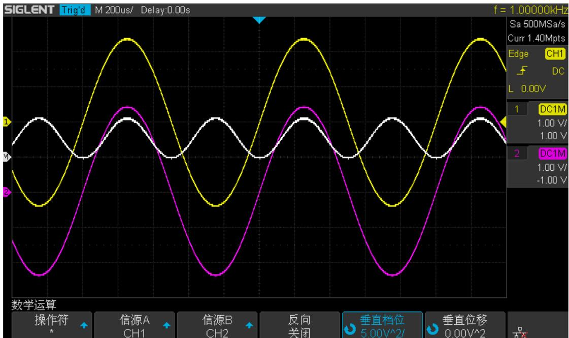
Figure 59 C1\*C2 Waveform
