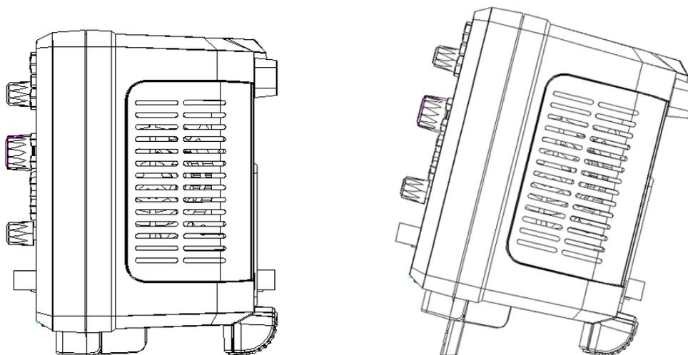
Figure 5 Adjust the Supporting Legs
