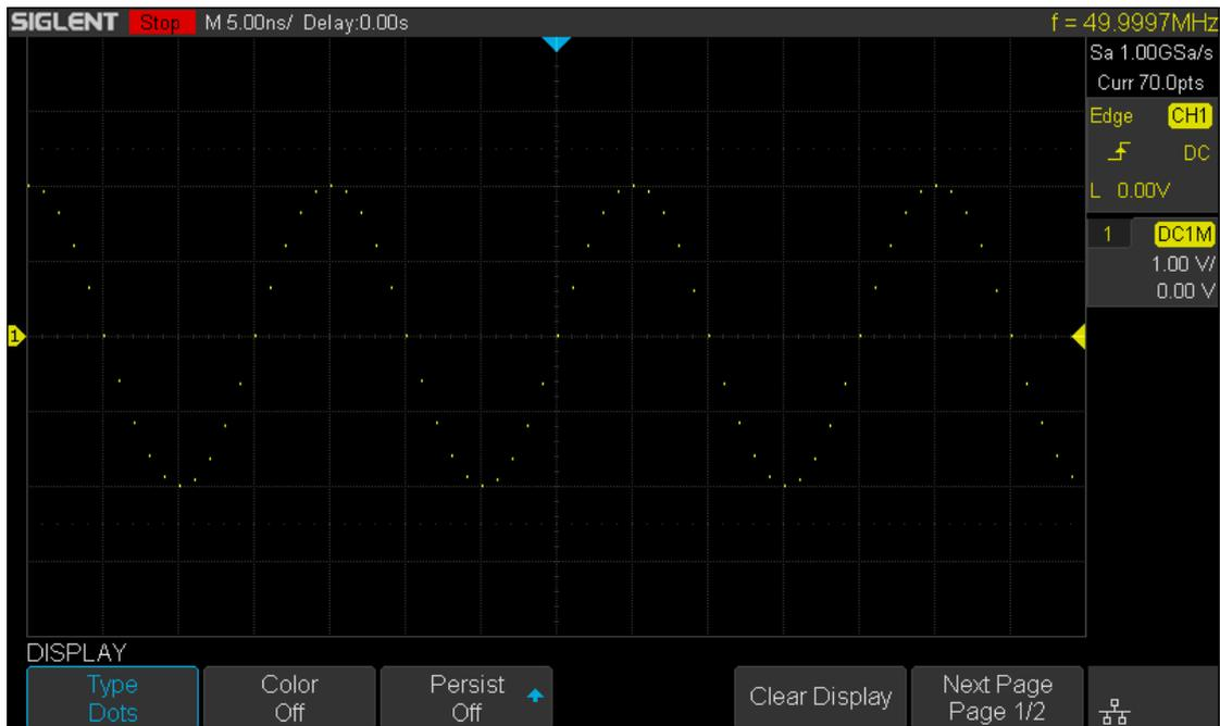
Figure 83 Dots Display
