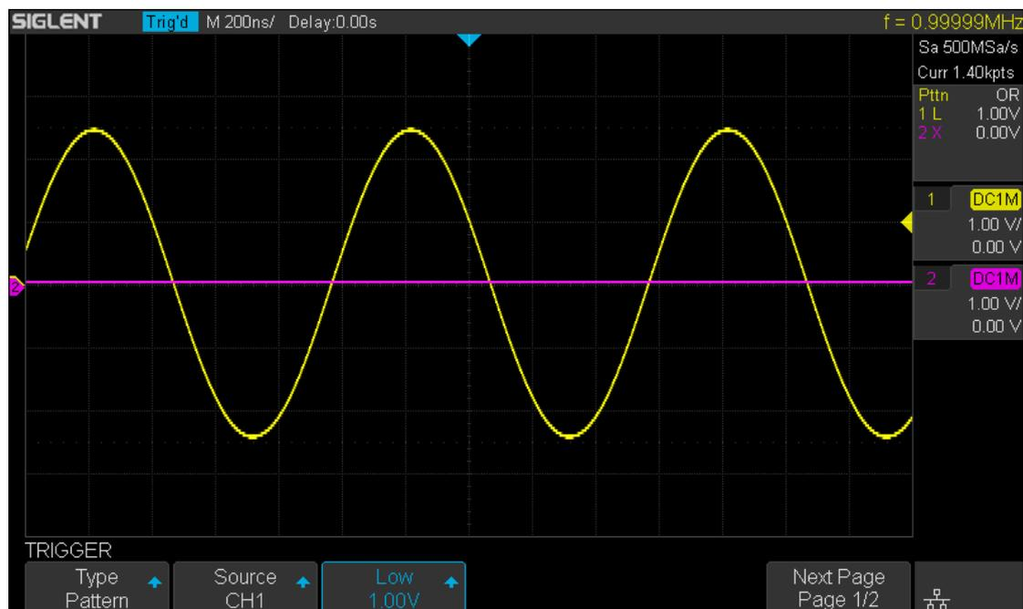
Figure 38 Pattern Trigger
