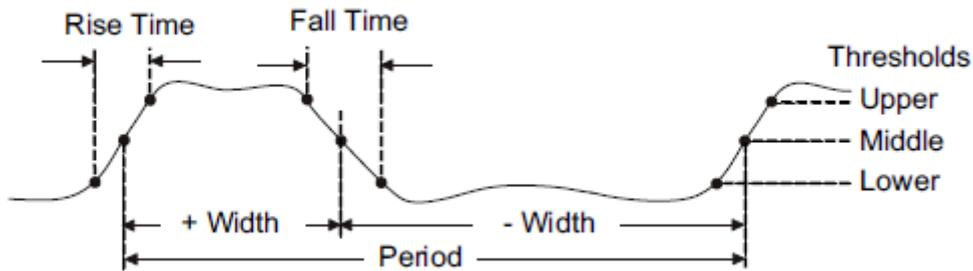
Figure 77 Time Measurements
