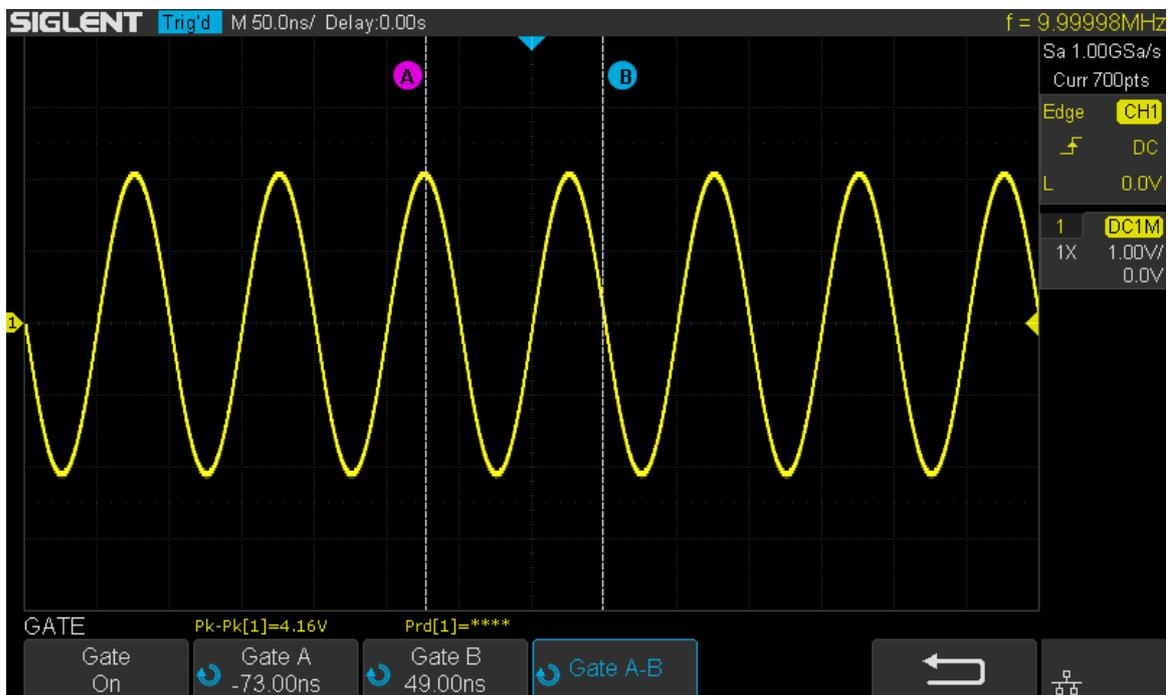
Figure 81 Gate Measurement
