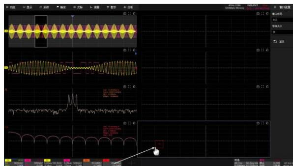
The instrument is able to automatically allocate a trace to a window according to the window layout and traces activated. If the user want to adjust the mapping relationship between a trace and a window, simply drag the Channel Descriptor Box of the trace to the destination window, as the right figure above shown. In this figure F2 is originally shown in window (4,1), to drag its channel descriptor box to window (4,2) will have the trace shown in window (4,2).
