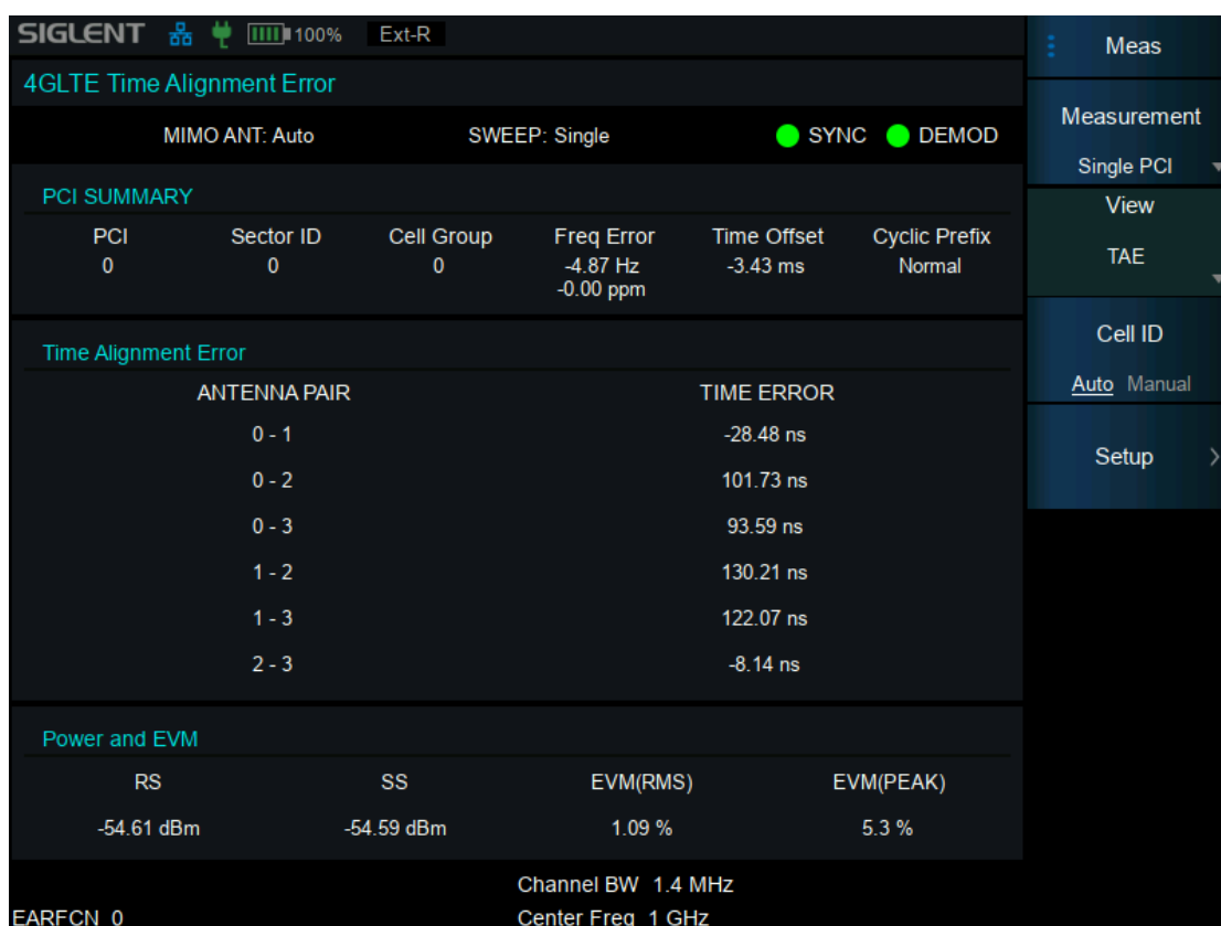
Figure 9–2 Single PCI TAE view
