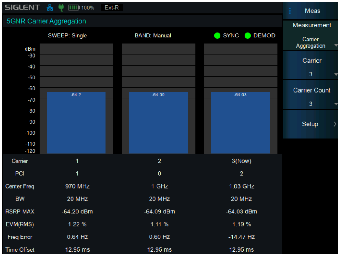
Figure 8–7 Carrier Aggregation View
