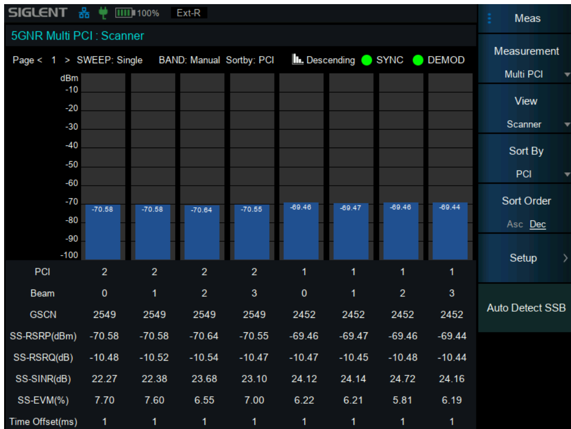
Figure 8–3 Multi-PCI histogram display
