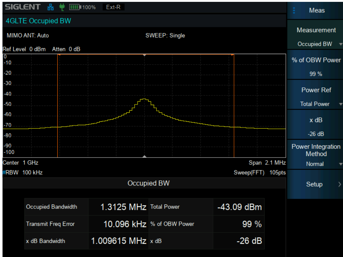
Figure 9–5 Occupied Bandwidth View
