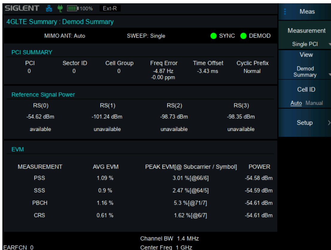
Figure 9–1 Single PCI Demodulation View
