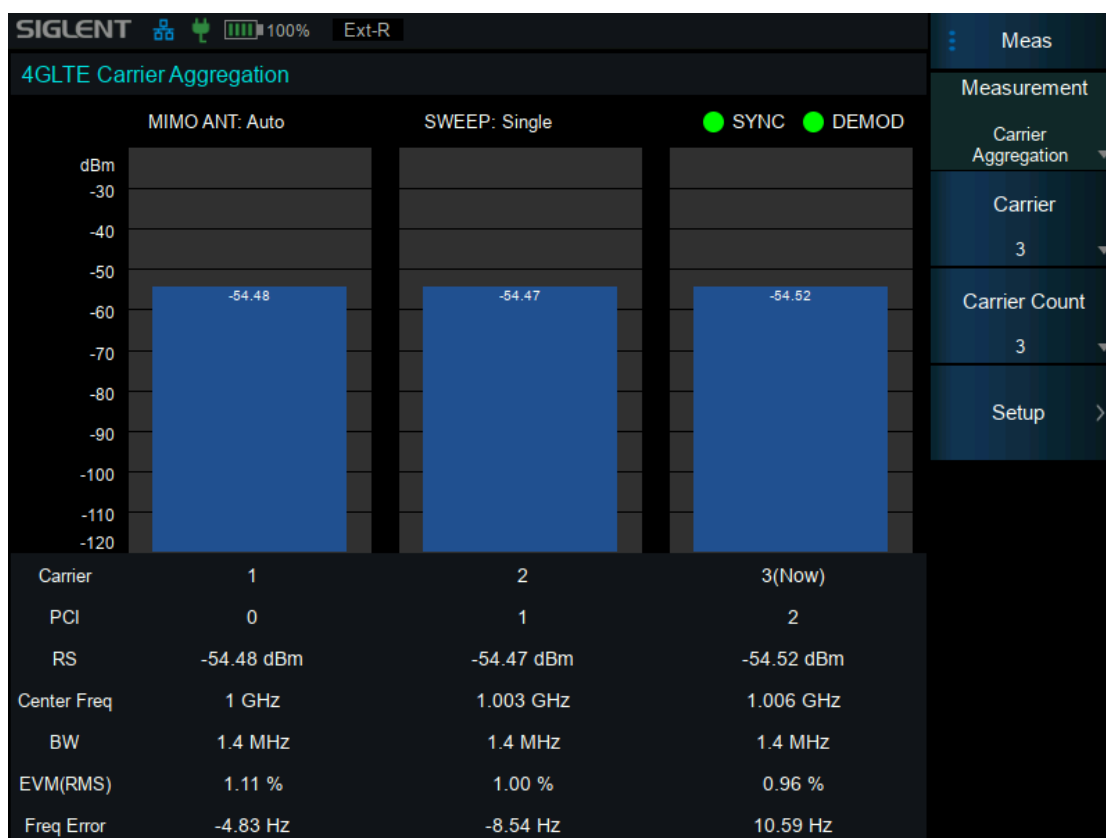
Figure 9–6 Carrier Aggregation View
