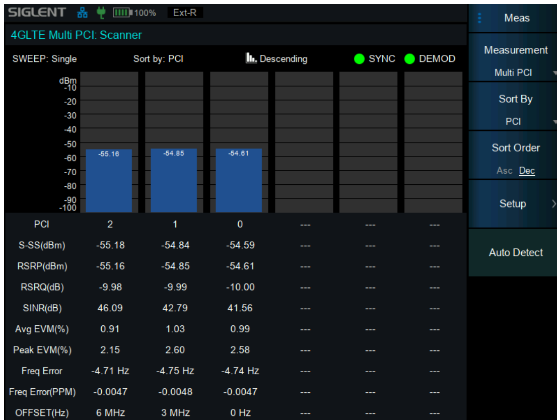
Figure 9–3 Multi PCI View
