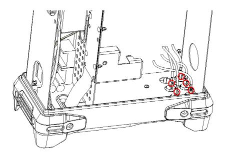
9. Remove the cable and unscrew all the screws,then you can remove the PCBA.
