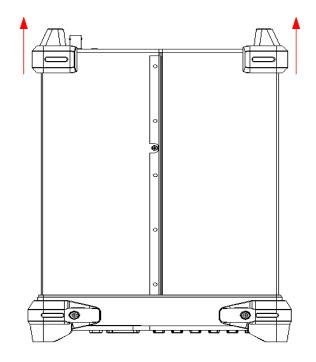
4. Remove the screw on the bottom of the instrument and place it in a safe location for re-assembly. Slide off the instrument cover as indicated by the arrow shown below.
