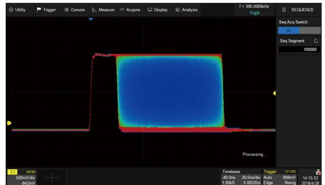
Segmented memory collection will store the waveform into multiple memory segments (up to 100,000) and each segment will store a triggered waveform as well the dead time information. The interval between segments can be as small as 2 μs. All of the segments can be played back using the History function
