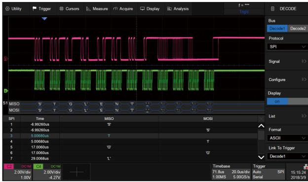
Display the decoded characters through the events list. Bus protocol information can be quickly and intuitively displayed in tabular form. I2C, SPI, UART, CAN, LIN, CAN FD, FlexRay, I2S and MIL-STD-1553B are supported
