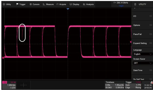
With a waveform update rate of up to 110,000 wfms/s, the oscilloscope can easily capture unusual or low-probability events. In Sequence mode the waveform capture rate can reach 500,000 wfms/s
