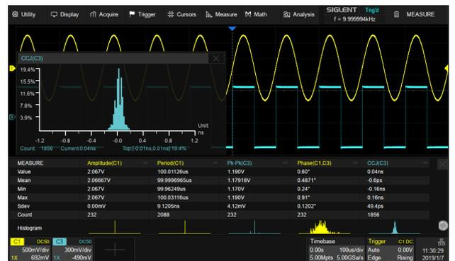
Statistics shows the current value, maximum value, minimum value, standard deviation and mean value of up to 5 parameters simultaneously. Histogram is available to show the probability distribution of a parameter. Trend is available to show the parameter value vs. time.
