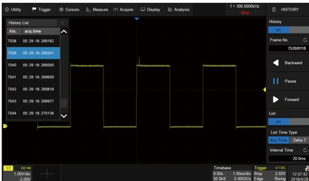
History function can record up to 100,000 frames of waveforms. The recording is executed automatically, so that the customer can play back the history waveforms at any time in order to observe unusual events and quickly locate the area of interest using the cursors or measurements
