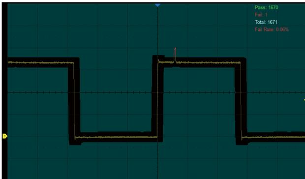
The SDS5000X utilizes a hardware-based Mask Test function, performing up to 18,000 Pass / Fail decisions each second. It is easy to generate user-defined test templates in order to provide trace mask comparisons, making it suitable for long-term signal monitoring or automated production line testing
