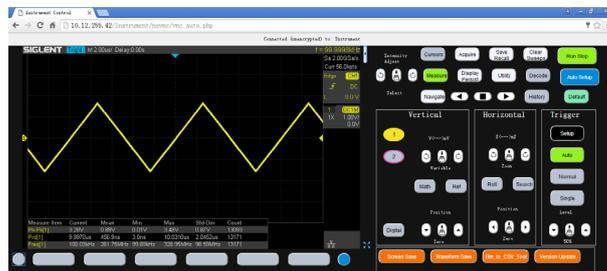
With the new embedded web server, users can control the SDS2000X-E from a simple web page. This provides wonderful remote troubleshooting and monitoring capabilities. The web page has PC and mobile styles that include an embedded virtual control panel.
