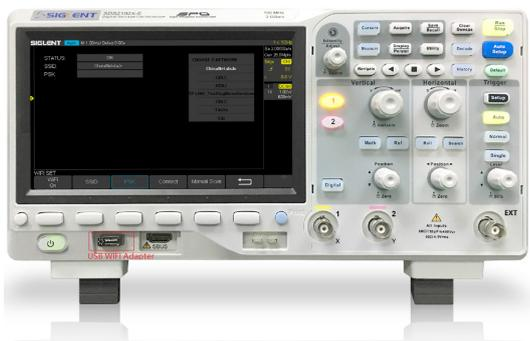
WiFi control of instrumentation can provide a convenient and safe method of configuring and collecting data. This new feature works with a SIGLENT approved WiFi adapter to provide wireless control and communications with SIGLENT SDS2000X-E scopes.
