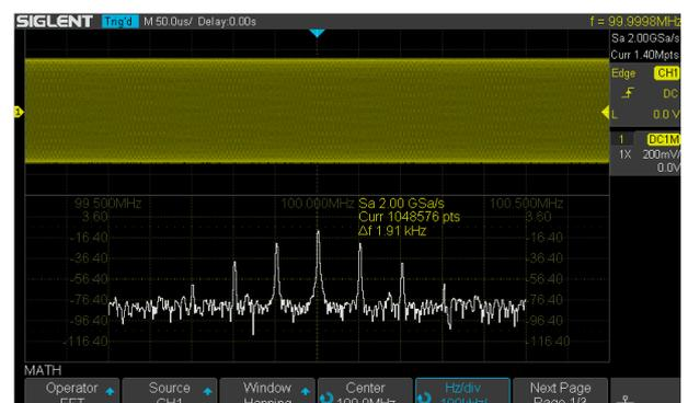
The new math co-processor enables FFT analysis of incoming signals using up to 1 million samples per waveform. This provides high frequency resolution with a fast refresh rate. The FFT function also supports a variety of window functions so that it can adapt to different spectrum measurement needs.
