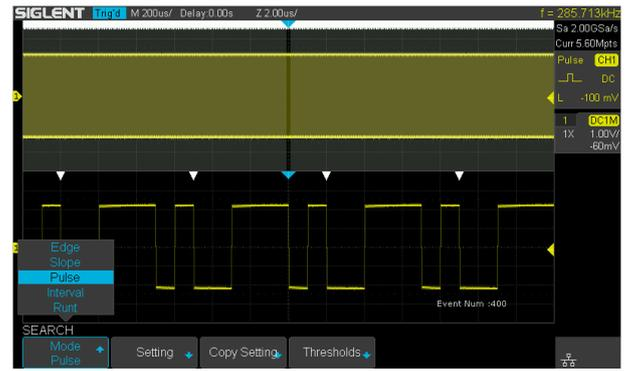
The SDS2000X-E can search events specified by the user in a frame. It can also navigate by time (delay position) and historical frames.
