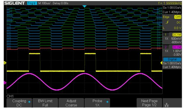
16 digital channels enables users to acquire and trigger on digital input channels and view both digital and analog waveforms simultaneously with one instrument.
