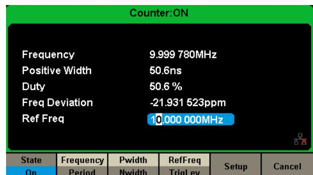
High precision Frequency Counter with an input frequency range of 0.1Hz~200MHz.
