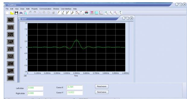
EasyWave is a powerful arbitrary waveform editing software that supports several ways to generate arbitrary waveform such as manual drawing, line-drawing, equation-drawing, coordinate-drawing, etc. It is quite convenient for users to edit their own arbitrary waveforms through EasyWave.
