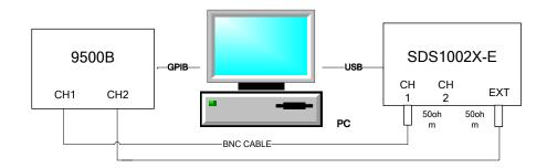
Figure 12 Connecting test instruments for Ext Trigger Delay
