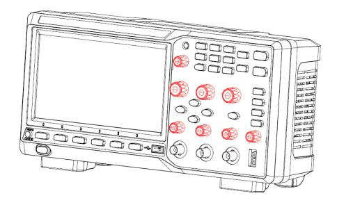
Figure 15 Removing the front panel knobs
