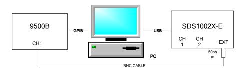
Figure 14 Connecting test instruments for Ext Trigger Sensitivity
