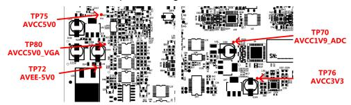
Figure 35 Test points for the Acquisition System power supplies section
