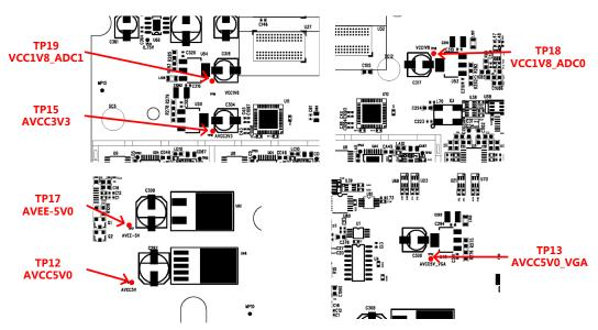
Figure 43 Test points for the Acquisition System power supplies section
