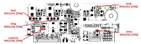
Figure 33 Test points for the processor power supplies
