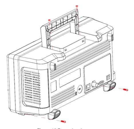
Figure 16 Removing the rear cover
