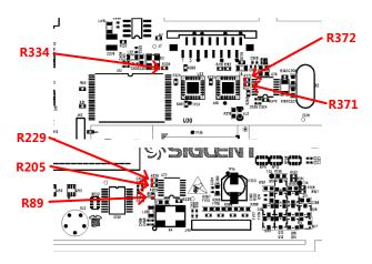
Figure 34 Test points for clock
