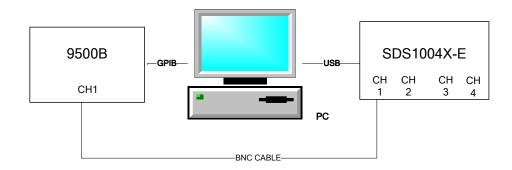
Figure 11 Connecting test instruments for Input impedance
