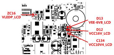
Figure 38 Test points for the LCD power supplies
