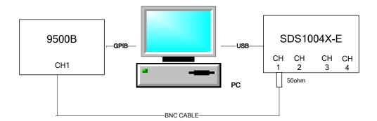
Figure 10 Connecting test instruments for BW\BWL\Trigger Sensitivity
