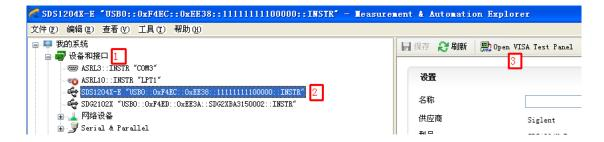
4. Click "Open VISA Test Panel" option button, and then the following Interface will appear. Next, click the "Input/Output" option button and click the "Query" option button in order to view the Read operation information.
