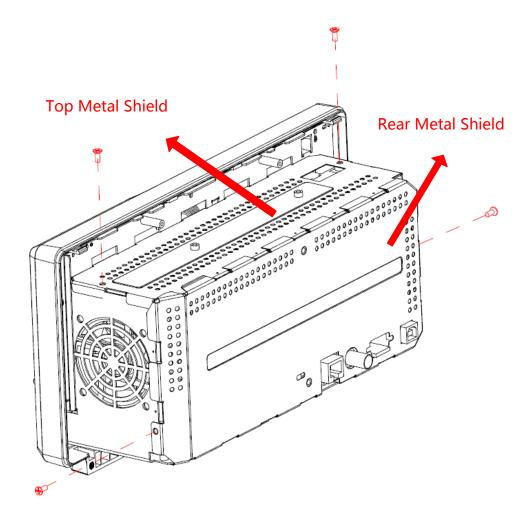
Figure 17 Removing the top and rear metal cover
