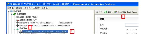
Click "Open VISA Test Panel" option button, which then displays the following interface (below). Then click the "Input/Output" option button and click the "Query" option button. The Read operation information will be displayed.
