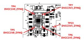
Figure 41 Test points for the processor power supplies
