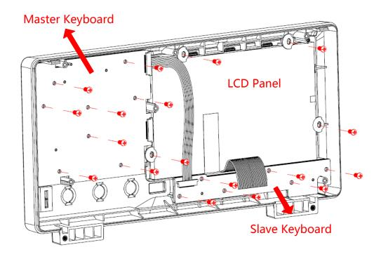
Figure 23 Removing the LCD panel and keyboard
