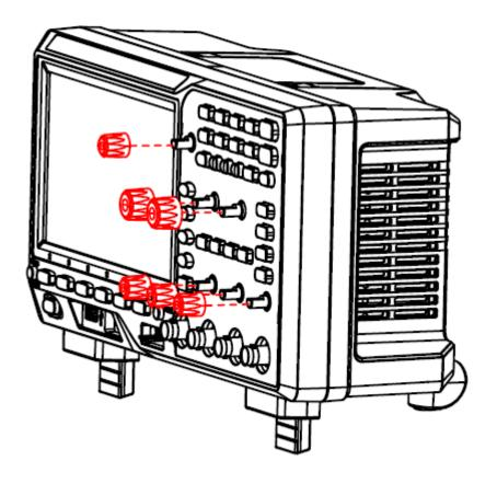
Figure 24 Removing the front panel knobs
