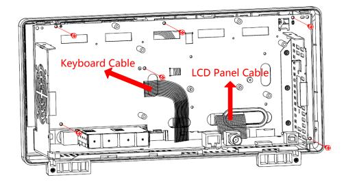
Figure 20 Removing the front cover
