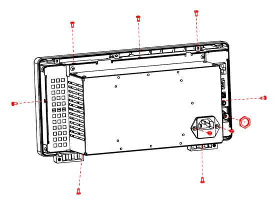
Figure 26 Removing the rear metal shield
