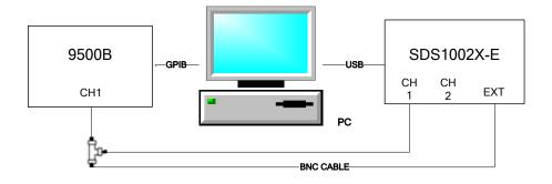
Figure 13 Connecting test instruments for Ext Trigger Level
