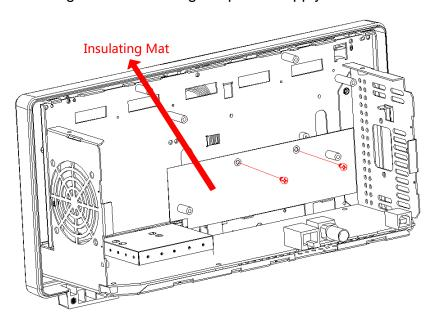
Figure 19 Removing the insulating mat
