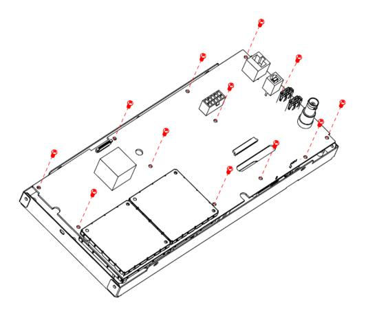
Figure 30Removing the main board
