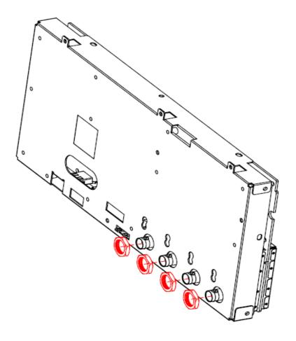
Figure 29 Removing the BNC nuts and gaskets
