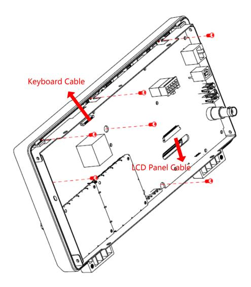
Figure 28 Removing the front cover
