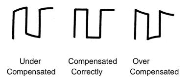
5. If the waveform does not show as "compensated correctly", use a nonmetallic screwdriver to adjust the low-frequency compensation adjustment hole on the probe until the waveform displays correctly.
