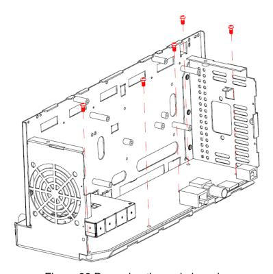
Figure 22 Removing the main board
