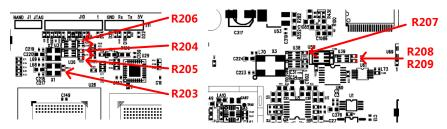
Figure 42 Test points for clock
