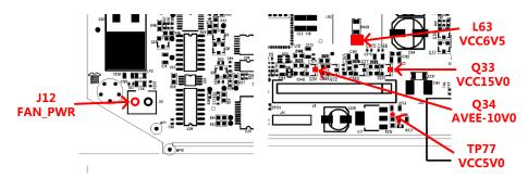
Figure 37 Test points for other power supplies
