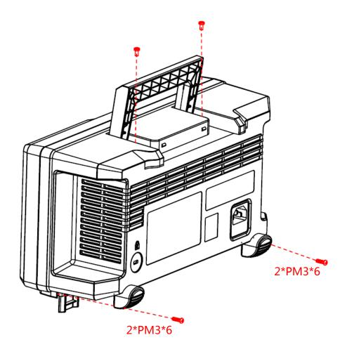
Figure 25 Removing the rear cover
