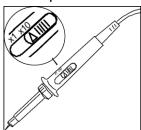
Figure 2 Set the attenuation switch
