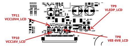
Figure 46 Test points for the LCD power supplies
