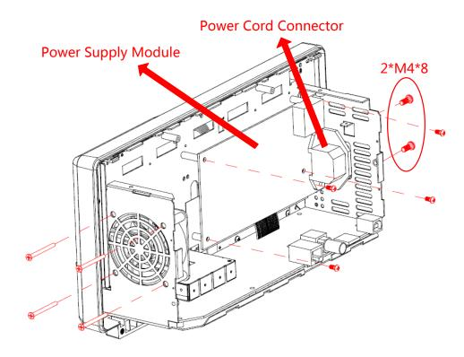
Figure 18 Removing the power supply module
