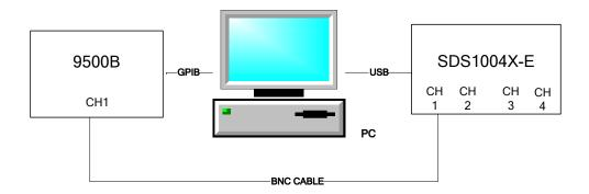
Figure 9 Connecting test instruments for Clock\Trigger Delay
