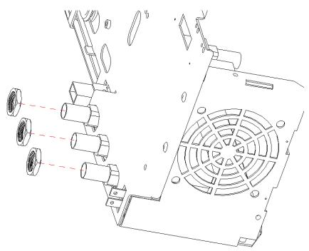
Figure 21 Removing the BNC nuts and gaskets
