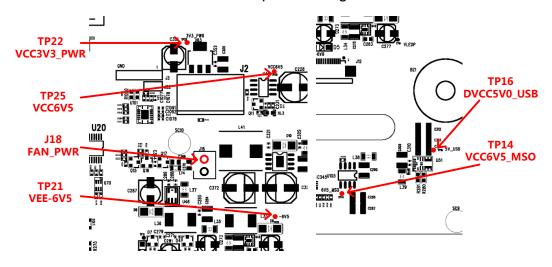
Figure 45 Test points for other power supplies
