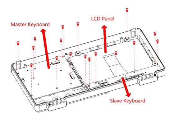
Figure 31 Removing the LCD panel and keyboard
