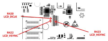
Figure 47 Test points for LCD signal
