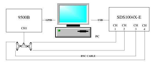
Figure 8 Connecting test instruments for DCG\Offset
