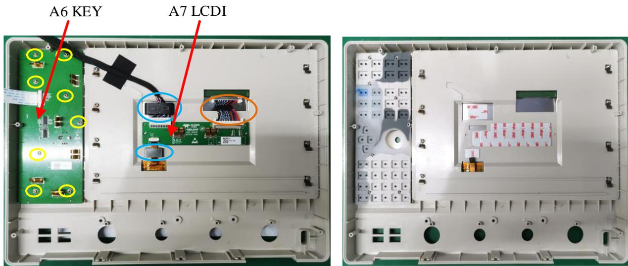
Figure 25 Diagram for removing A6, A7.
