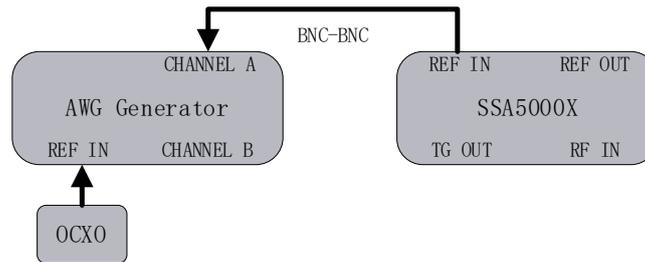
Figure 15 Diagram of Frequency Accuracy Test System
