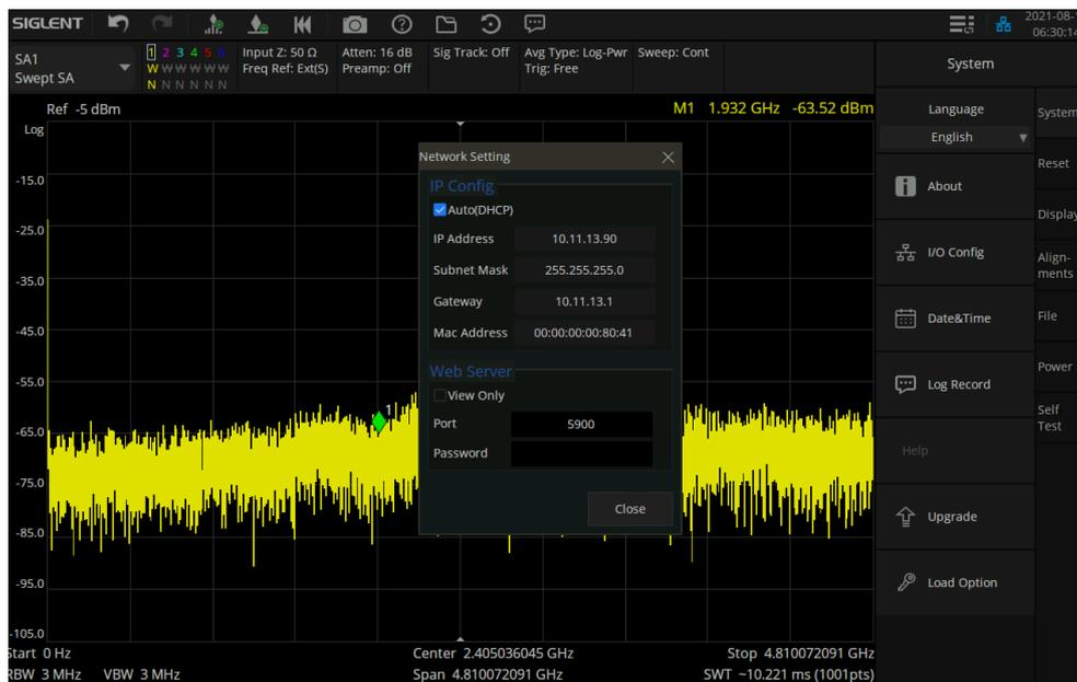
Figure 3 IP configuration interface
