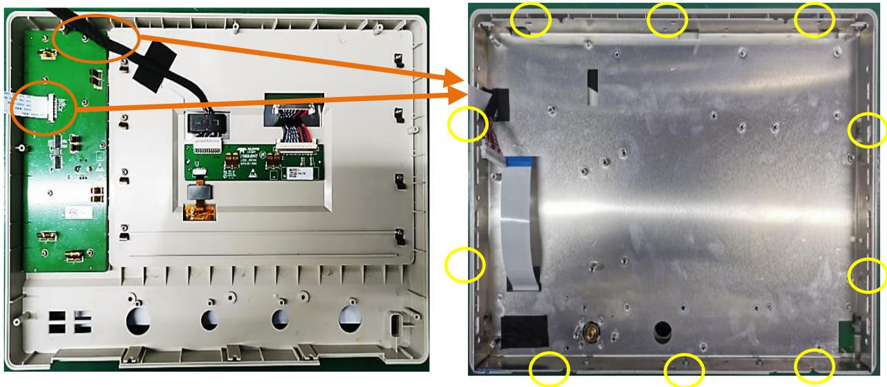
Figure 24 Diagram for removing front metal cover.
