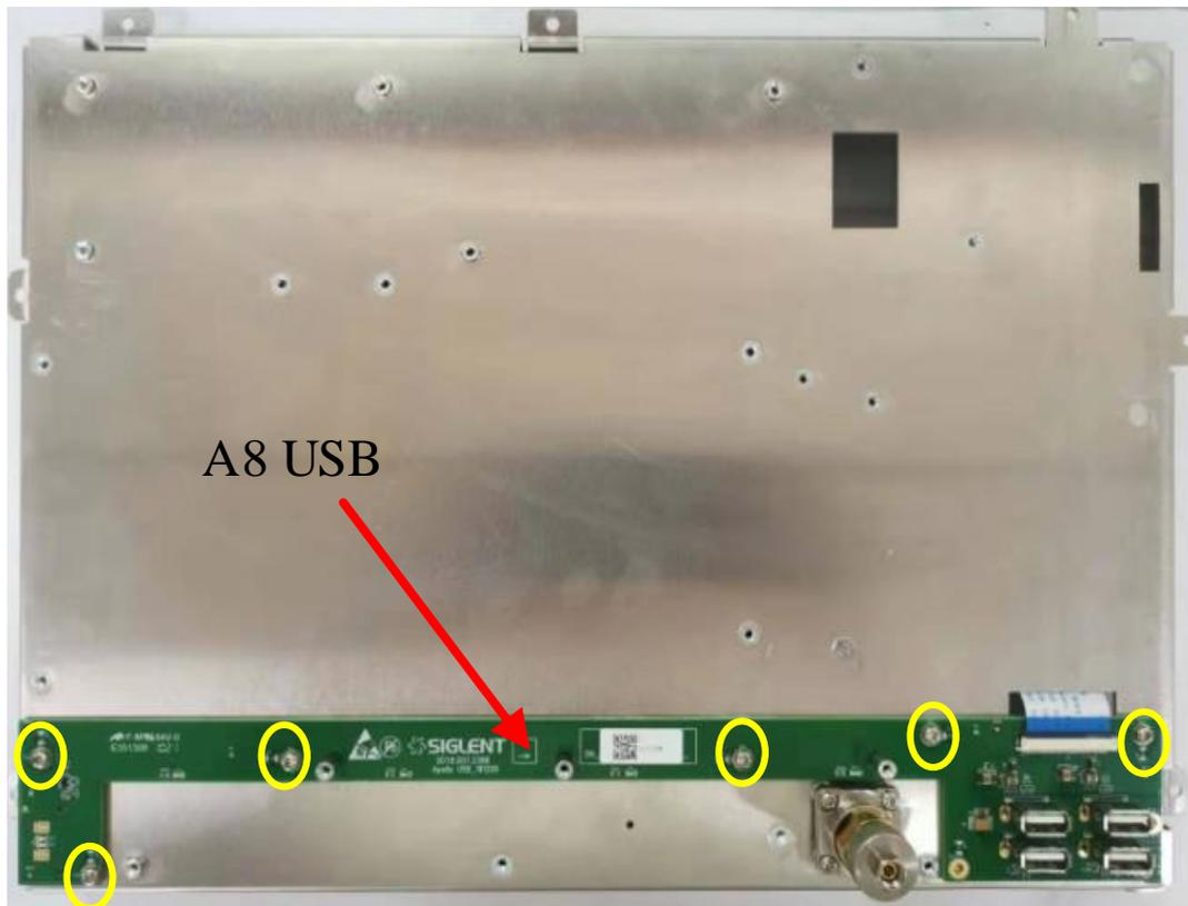
Figure 26 Diagram for removing A8.
