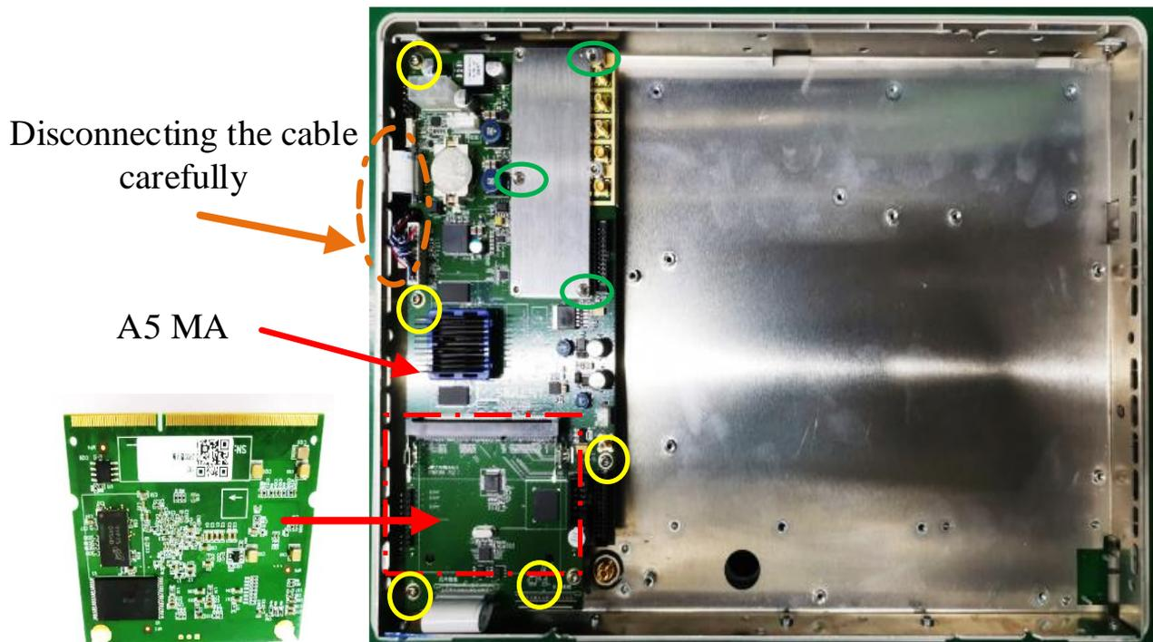
Figure 23 Diagram for removing A5
