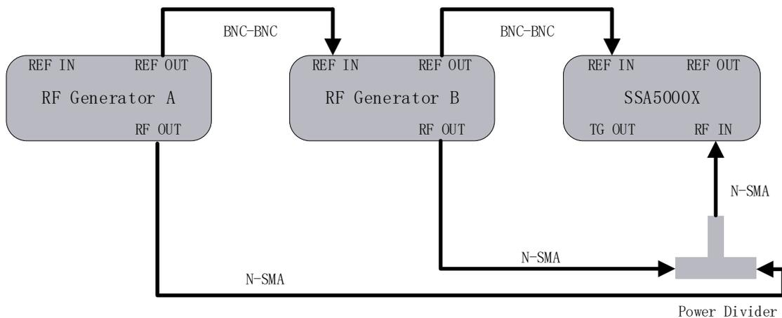
Figure 14 Diagram of TOI Test System
