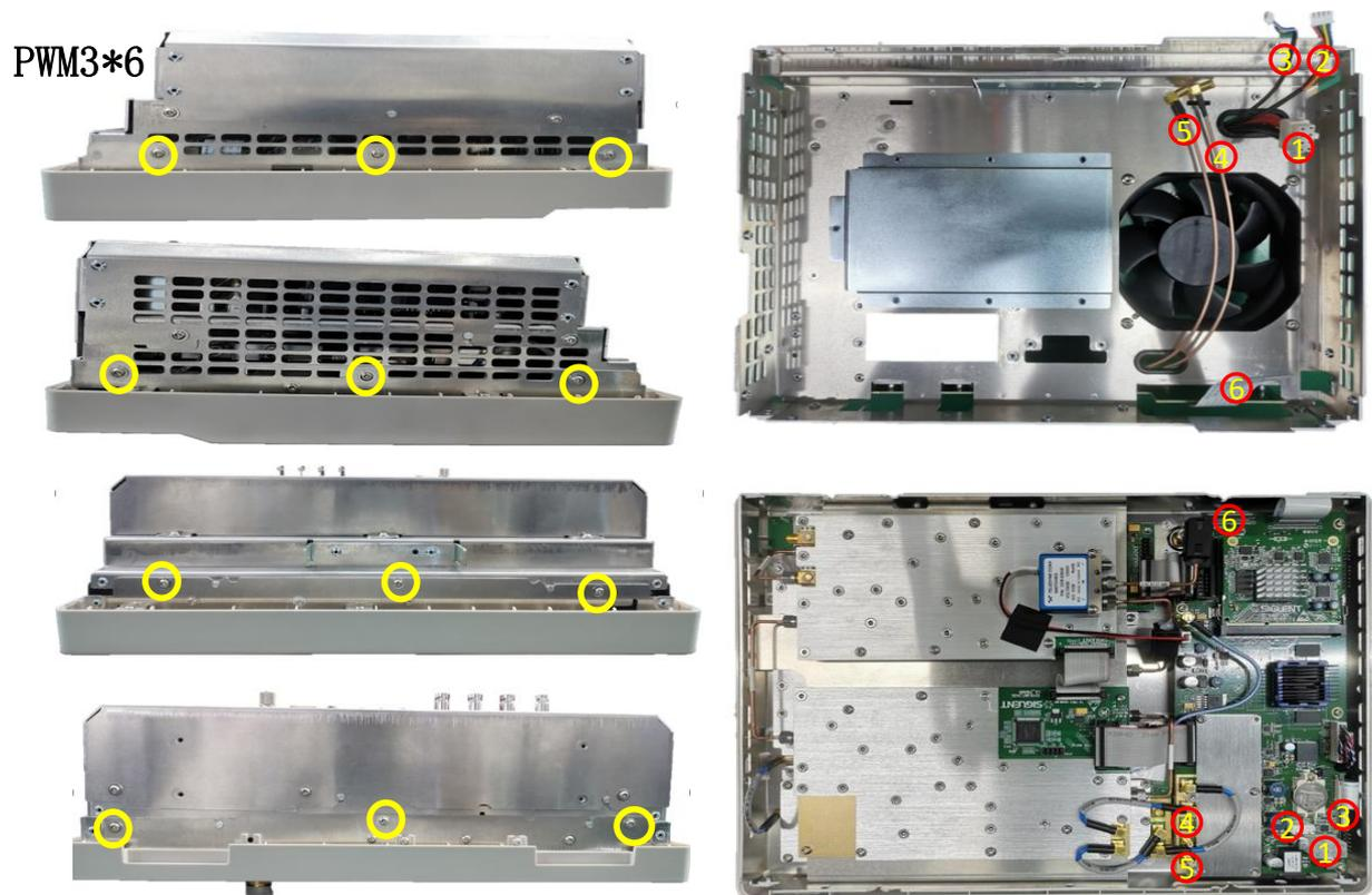
Figure 21 Diagram for removing rear metal cover.
