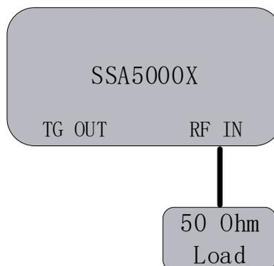
Figure 12 Diagram of DANL Test System
