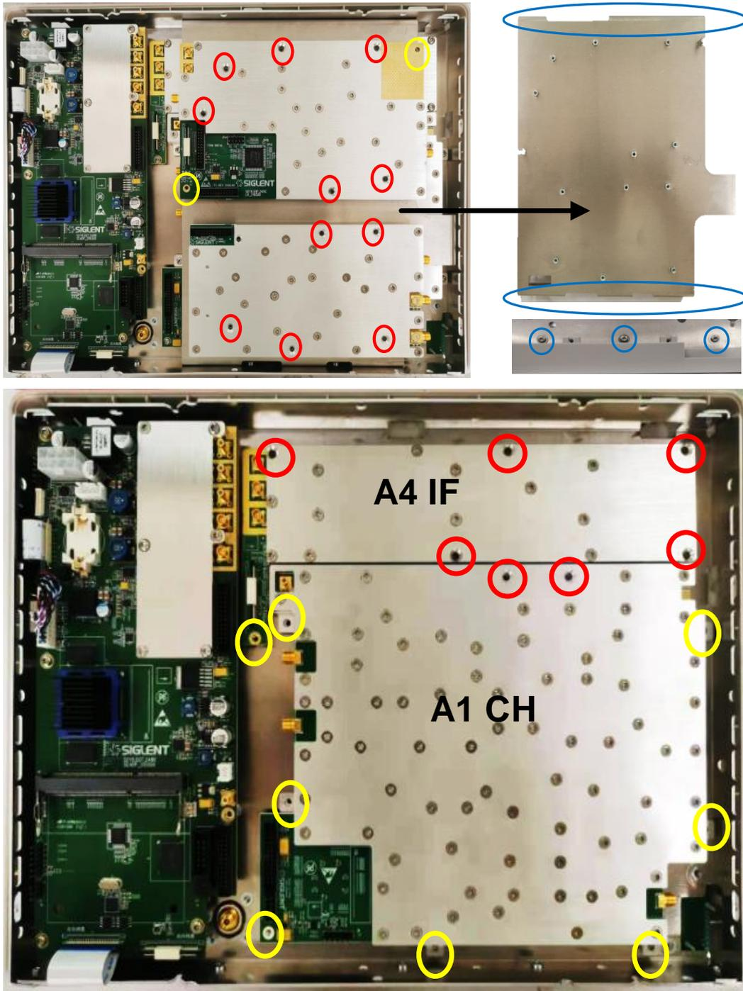
Figure 22 Diagram for removing A1, A2, A3, A4.
