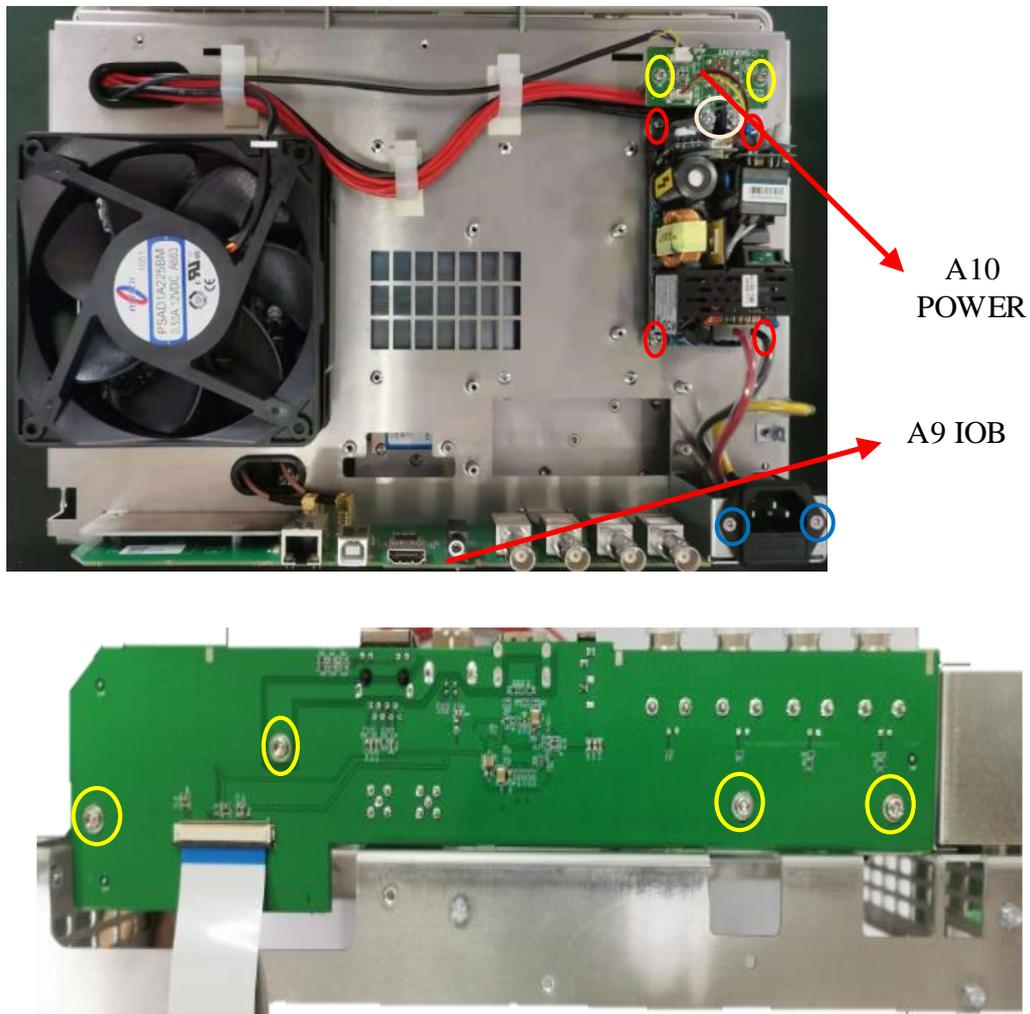
Figure 27 Diagram for removing A9, A10.
