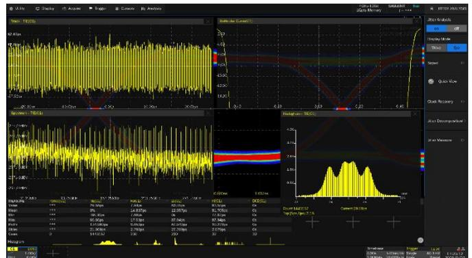
Supports eye diagram and jitter analysis/measurement. It can automatically extract the embedded reference clock from serial data and create the eye diagram. Measurement on multiple eye/jitter parameters is provided. Mask test on eye diagrams is supported
