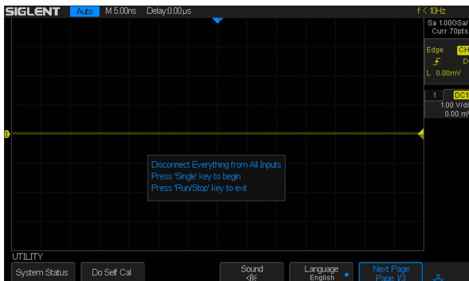
Figure 2-3 Calibration interface
