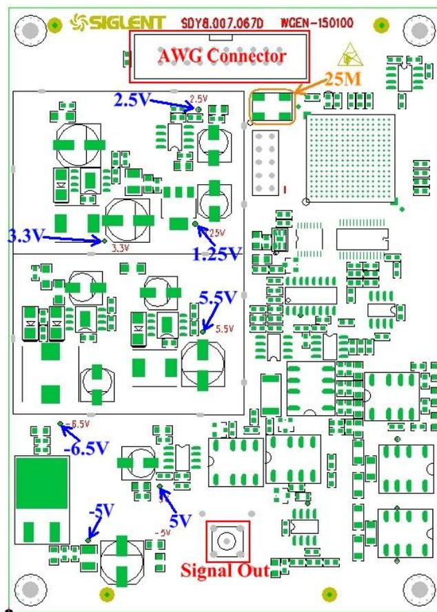
Figure 6-2 AWG board module
