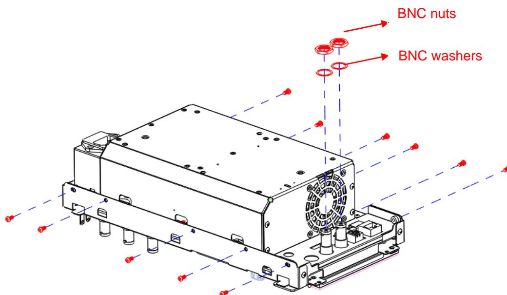
Figure 5-4 Removing the rear metal cover
