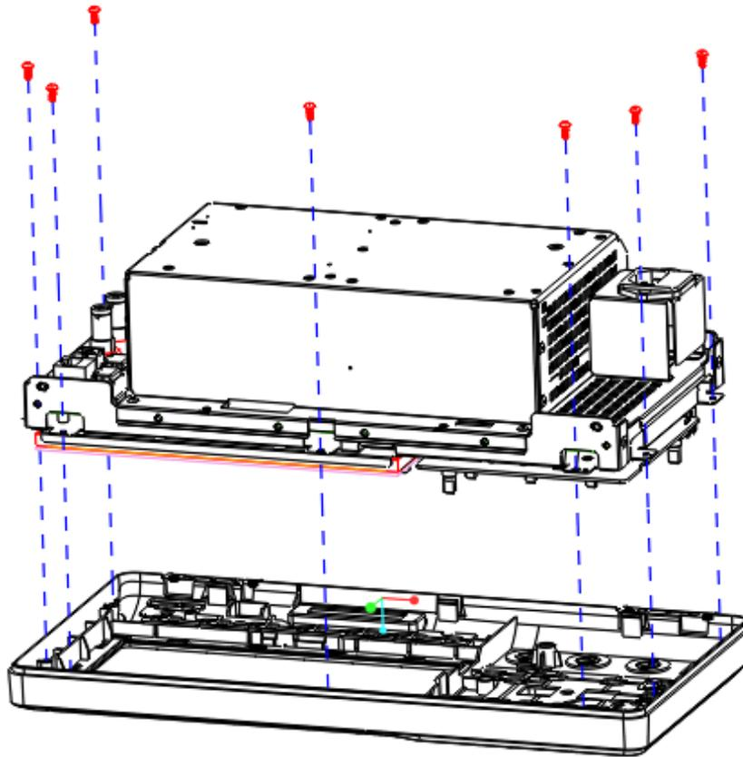
Figure 5-3 Removing the front panel
