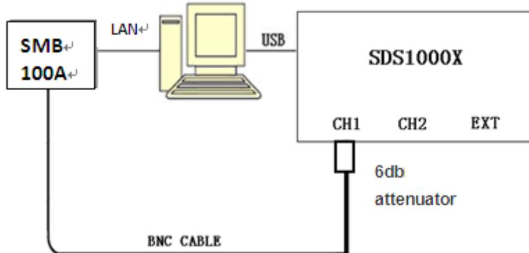
Picture 3-4 Connecting test instruments for BW\BWL\ Trigger Sensitivity
