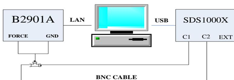
Picture 3-1 Connecting test instruments for DCG\Offset
