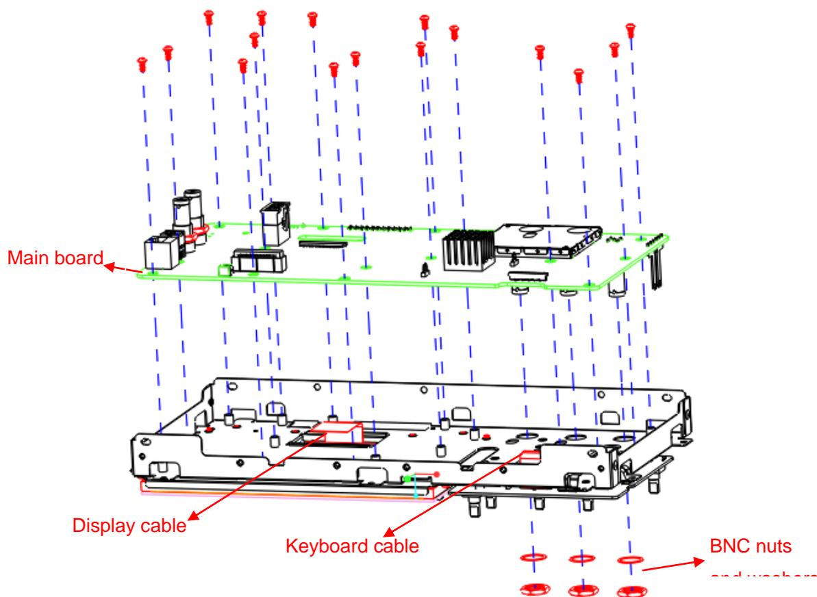
Figure 5-8 Removing the main board
