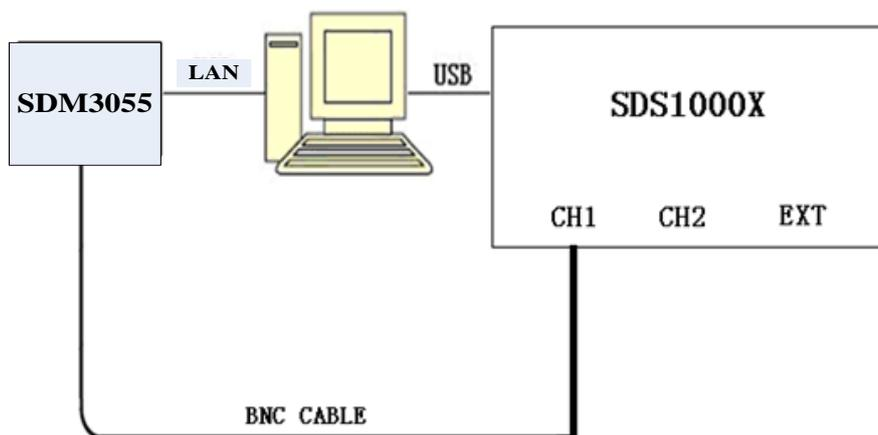
Picture 3-5 Connecting test instruments for Input Impedance
