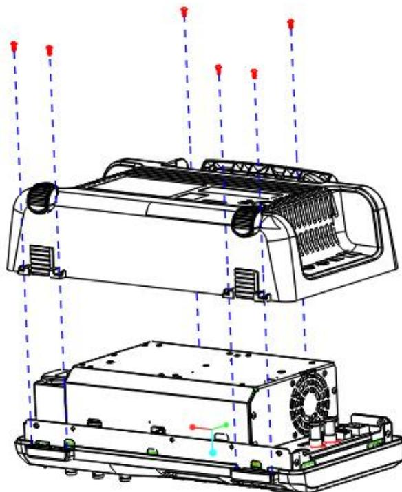
Figure 5-2 Removing the rear panel
