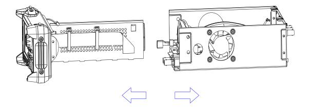
5. Pull out the knob and then remove the screws attaching the hardware partition plate and the front cabinet screws.
