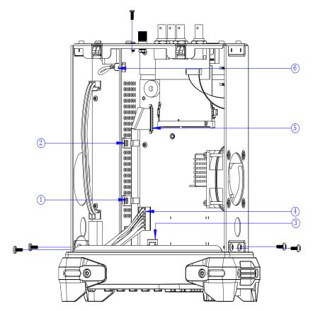
4. Separate the front panel from the main body of the generator.
