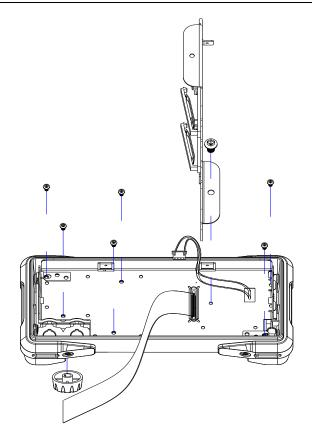
6. Remove the keypad circuit board assembly.
