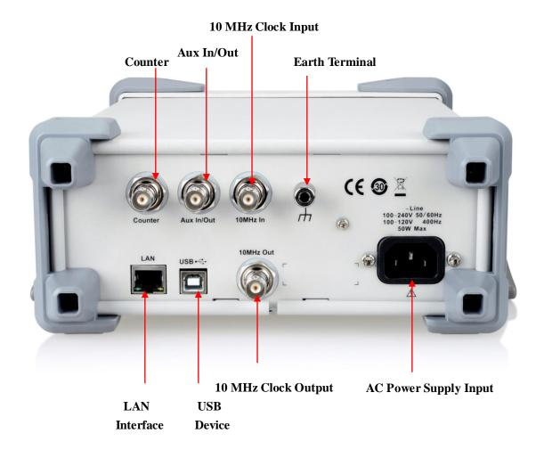
**WARNING:** For protection from electric shock, the grounding power cord must not be defeated. If only a two-contact electrical outlet is available, connect the instrument's chassis ground screw (see above) to a good earth ground.
