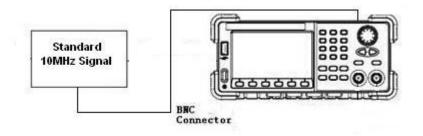
2. Press Utility button on the front panel and select System  $\rightarrow$  Page 1/2  $\rightarrow$  System Info. Use the number keyboard to input "123654". Then select the TimeBase Calibration softkey. The timebase calibration interface is shown as the following.
