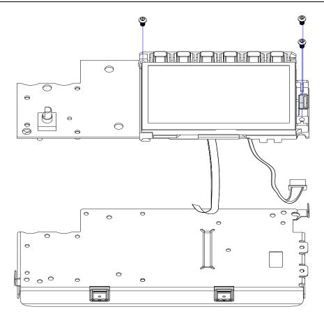
8. Pull out the connecting cable according to the index number as shown in the following figure and remove the keyboard.
