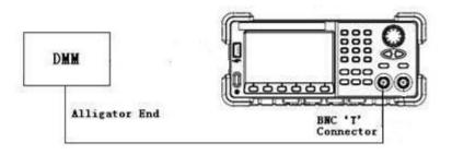
3. Select a 10 kHz Sine waveform of the generator and set the amplitude to the values listed below in sequence.
