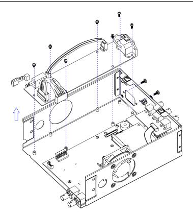
10. Pull out the connecting cable as shown in the following figure and then remove the fan, rear interface board, channel board and main board.
