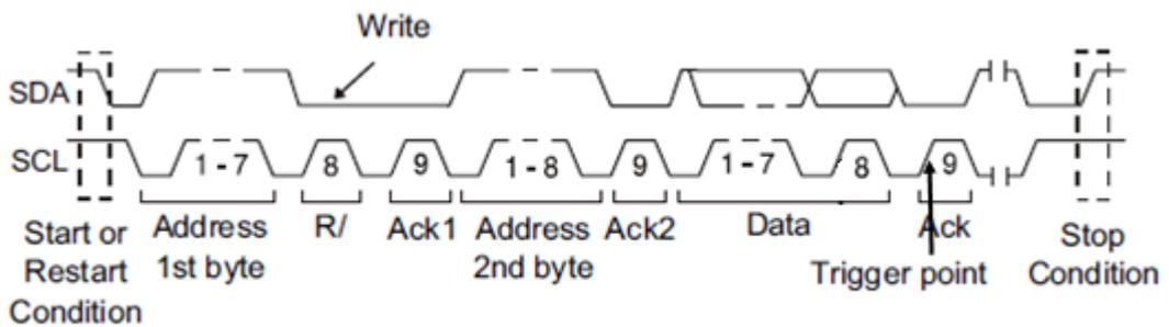
If you set the trigger condition to 7 address & data or 10 address & data:
