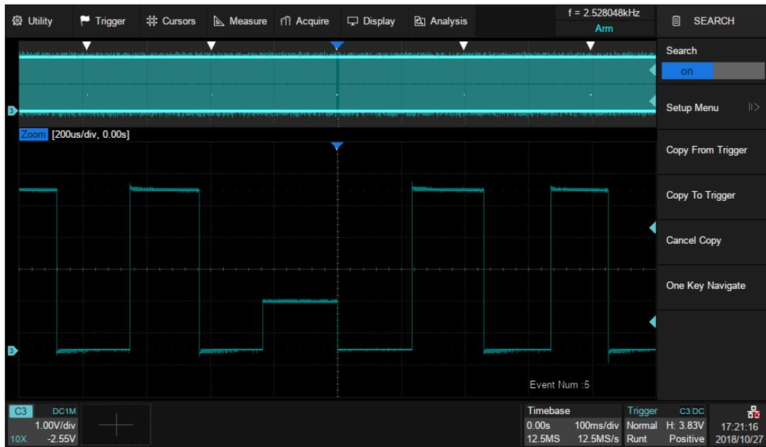
Press the **Run/Stop** button on the front panel to stop the acquisition, and then follow the steps **Navigate** > **Type** to select “Search Event”. The following figure shows the first dwarf pulse. In this example the list is enabled and time labels of each event are shown in the list.
