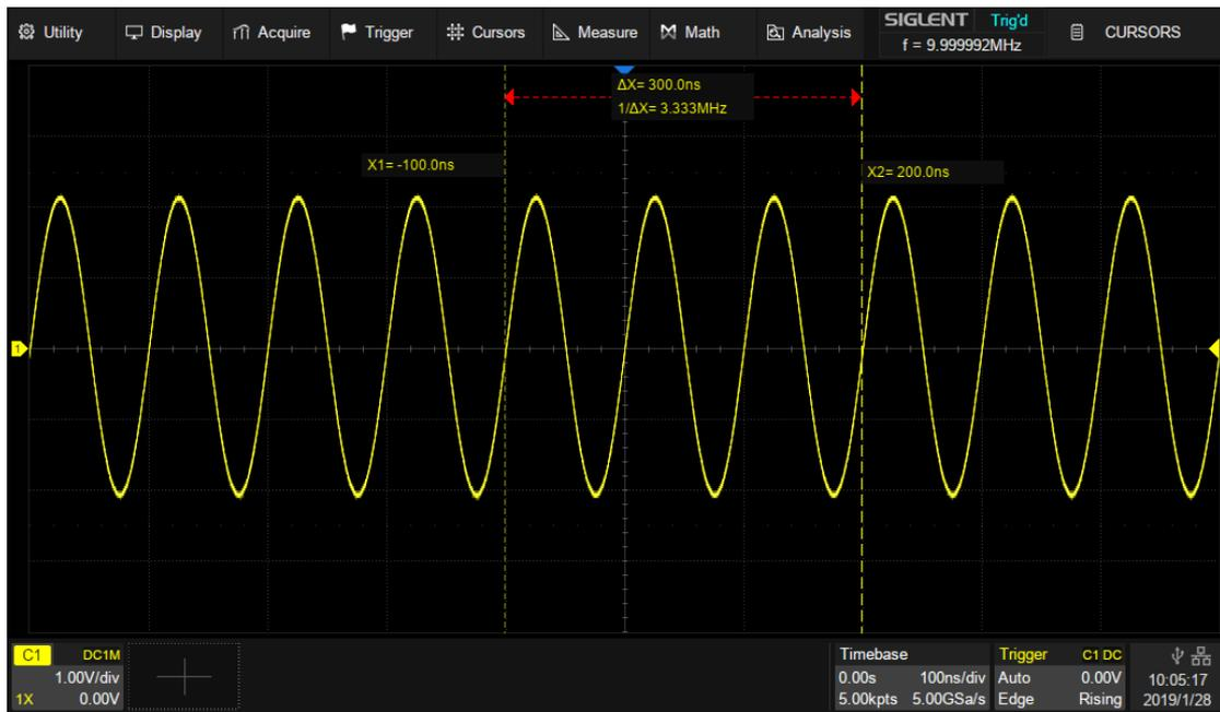
Fixed position, timebase is changed to 100ns/div, the grid number of X cursors (-1div, 2div) remains fixed. The value of X1 and X2 are changed to -100ns, 200ns.
