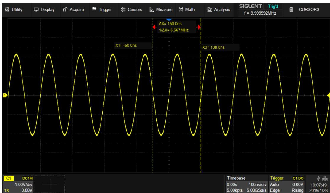
Fixed delay, timebase is changed to 100ns/div, the value of X cursors (-50ns, 100ns) remains fixed. The grid number of X cursors are changed to -0.5div, 1div.
