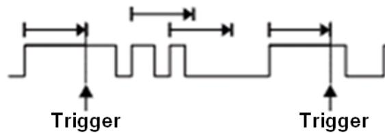
Trigger source, slope (rising, falling), dropout type and time value can be set in the trigger dialog box. Holdoff, coupling and noise reject can be set in dropout trigger, see the sections " Holdoff", " Trigger Coupling" and " Noise Reject" for details.
