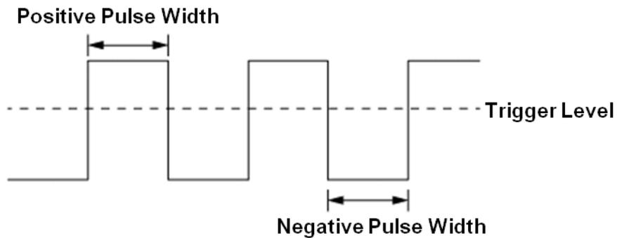
**Less than a time value ( $\leq$ )** -- Trigger when the positive or negative pulse time of the input signal is lower than the specified time value. Below is an example of trigger condition is set to positive pulse width  $< 100\text{ns}$
