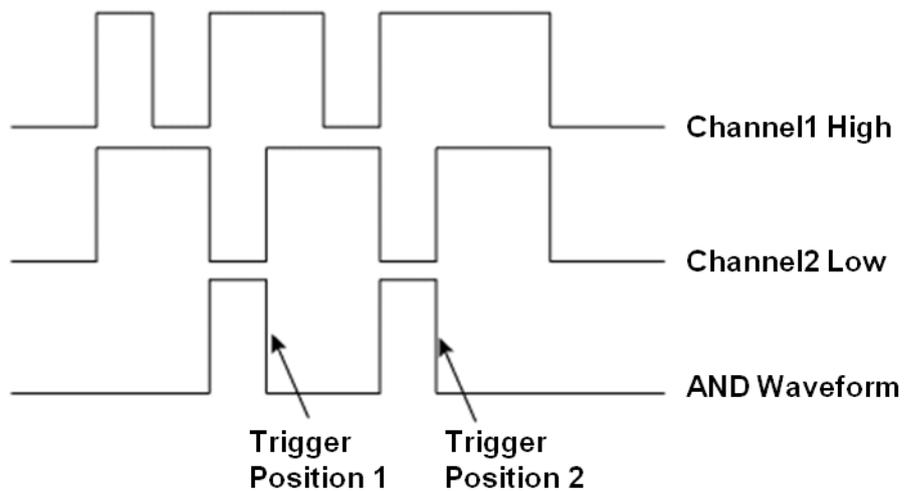
Logic (AND, OR, NAND, NOR), source, limit range and time value can be set in the trigger dialog box. When the logic is "OR" or "NAND", the setting of time limit is invalid.
