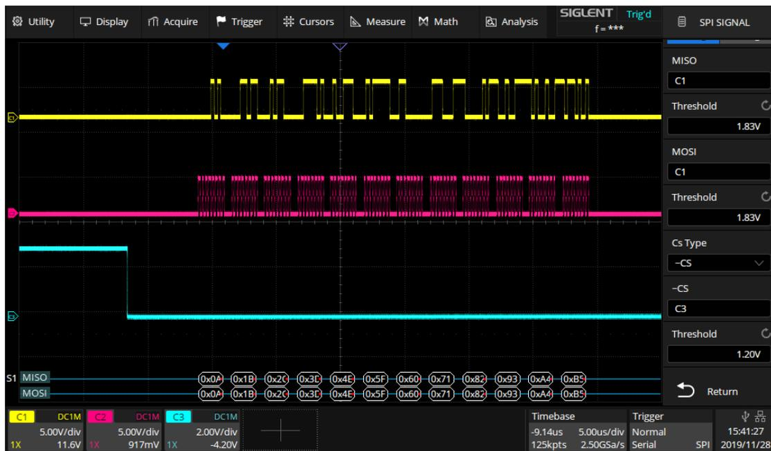
When the CS type is set to Clock Timeout, turn on Cursor, measure the clock idle time between frames as 150 us, and measure the interval between clock pulses as 0.14 us, then set the timeout to a value between 0.14 and 150 us. In this example it is set to 500 ns:
