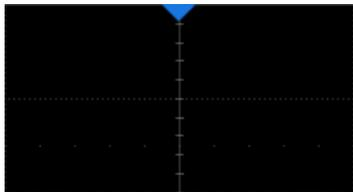
**Trigger Delay Indicator** locates where the waveform triggers on the horizontal axis...
