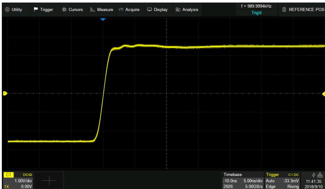
Fixed position, timebase is changed to  $5\text{ns/div}$ , the grid number of delay ( $-2\text{div}$ ) remains fixed, while the horizontal delay changes to  $-10\text{ns}$
