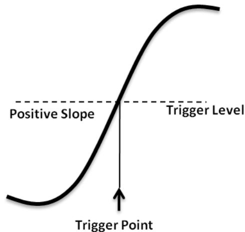
In some special trigger, the system will automatically set the trigger level, such as using AC Line as the trigger source.
