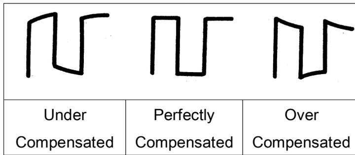
5. Use a non-metallic driver to adjust the low-frequency compensation adjustment hole on the probe until the waveform displayed is as the “Perfectly compensated” in the figure above.
