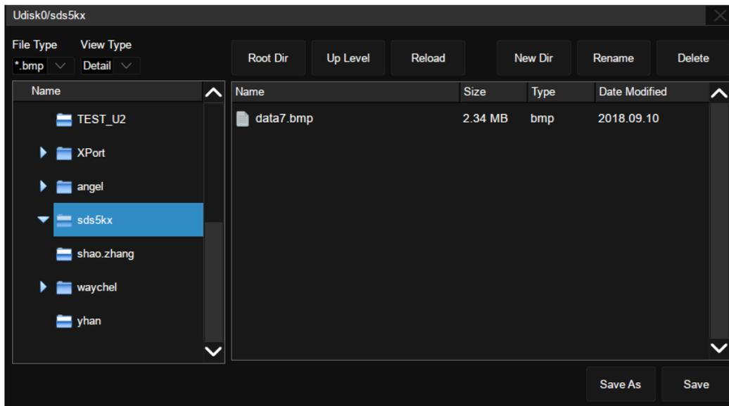
In step 4, if **Save** is selected instead of **Save As**, the system saves the file as the default file name sds5000x\_n.bmp, where n is an integer incrementing from 1. The default save path is \SIGLENT\.
