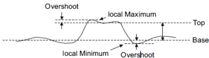
$$\text{Rising Edge Overshoot} = \frac{\text{Maximum} - \text{Top}}{\text{Amplitude}} \times 100\%$$
