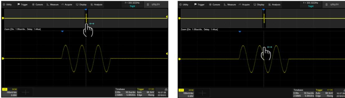
Adjust the horizontal position of the zoom area by dragging left and right in the zoom area of the main window or waveform in Zoom window
