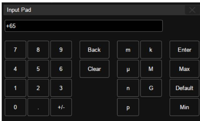
Let's use the operation of setting the "deskw" of a channel as an example: If the expected value is 65 ns, input "65" on the virtual keypad, and then choose the unit **n** to complete the operation. On the virtual keypad, touching the button **Max**, **Min**, and **Default** quickly sets the parameter to its maximum, minimum and default values.
