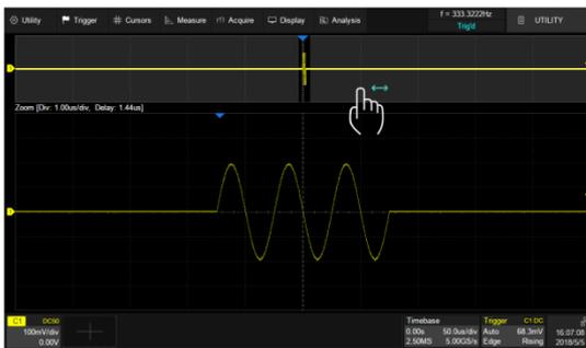
Adjust the horizontal position of the waveform by dragging left and right in the gray area of the main window
