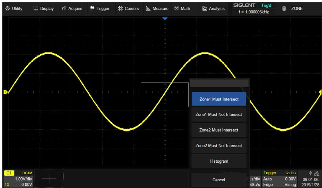
Once a zone is created, it can be moved by dragging. Just touch and hold the zone box and use a dragging gesture.
