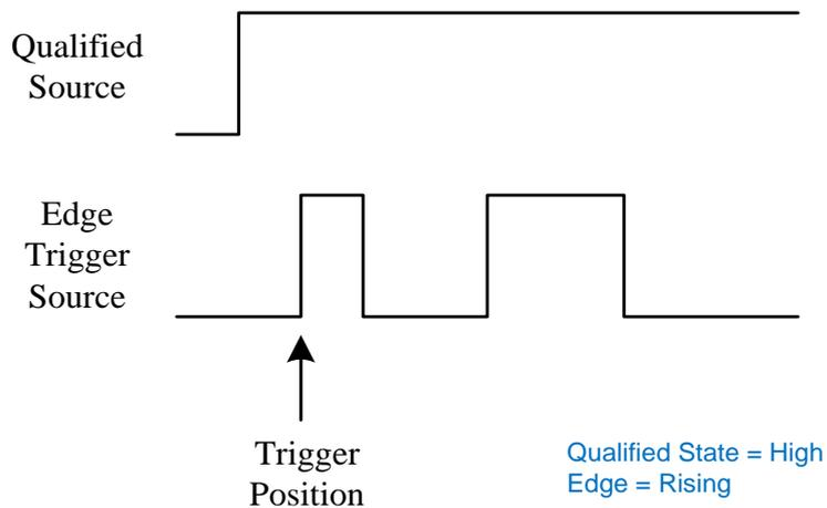
When the type is “Edge”, the oscilloscope triggers at the first edge after the specified edge (Rising or Falling) of the qualified source; when the type is “Edge with Delay”, time limit condition is available.
