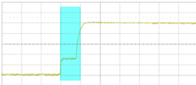
With a simple edge trigger, it is unlikely to trigger consistently on this anomaly. Thanks to the high waveform update rate of the SDS5000X, we can confirm
