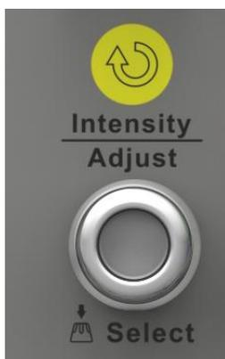
When the parameter setting area is highlighted, you can use the Universal Knob to adjust or set the parameter. Press the knob to select an option from the list. The default function of the Universal Knob is to adjust intensity of the waveform traces.
