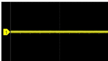
**Channel Offset Indicator** with a channel number shows the offset position of the corresponding channel.
