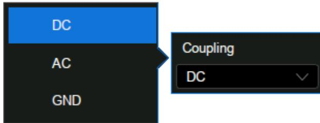
**List:** Sets parameters with more than two options, such as coupling mode of channels. Touch the parameter region, and then select the expected option from the pop-up list.
