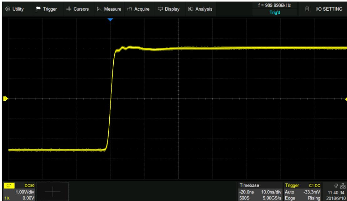
Timebase= $10\text{ns/div}$  , Horizontal Delay= $-20\text{ns}=-2\text{div}$
