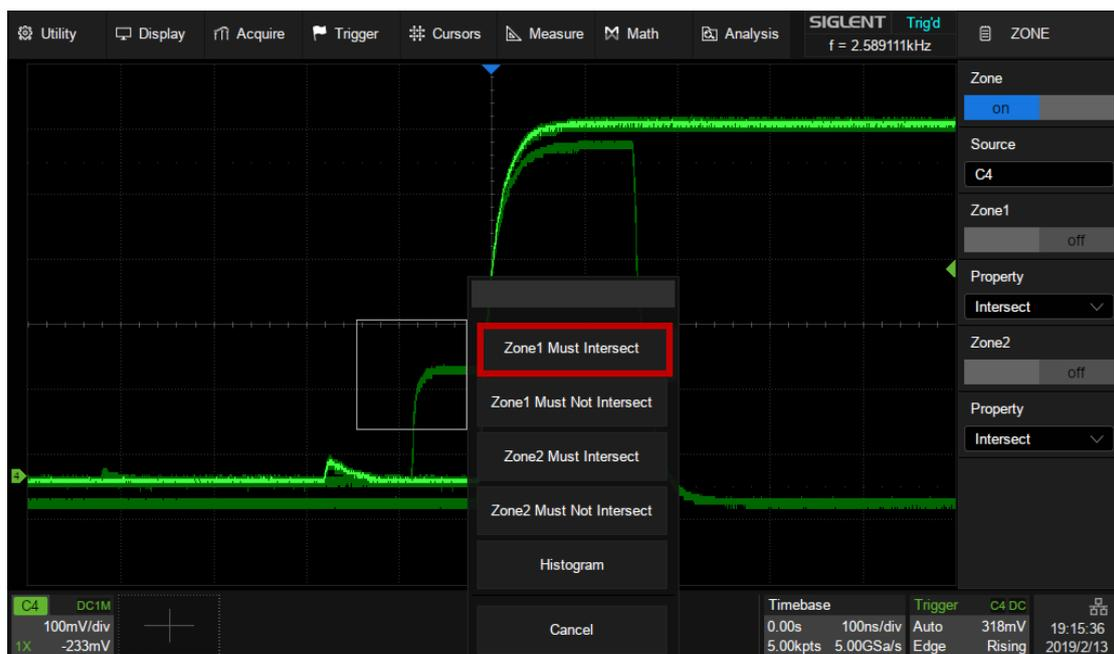
Now, we can accurately capture the exact bus contention waveform:
