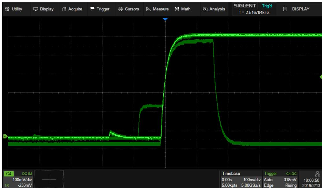
In this case zone trigger is a quick and simple way to capture the interested waveform. Enable the zone trigger, and draw a box to intersect with the bus contention part, as shown in the figure below:
