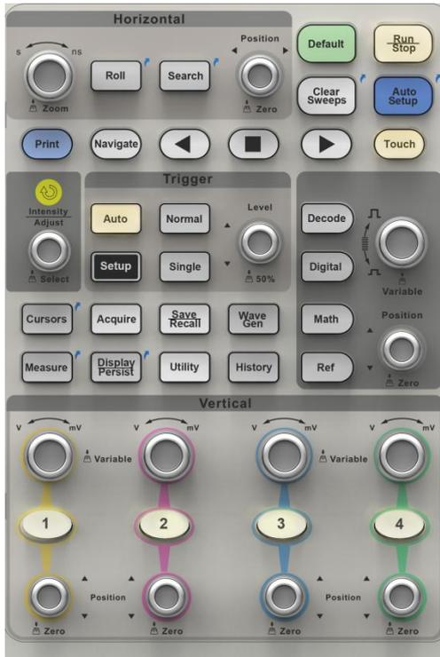
The front panel is designed to operate the basic functions without having to open the software menu. Most of the front panel controls duplicate functionality available through the touch screen display but the operation is more quickly achieved.
