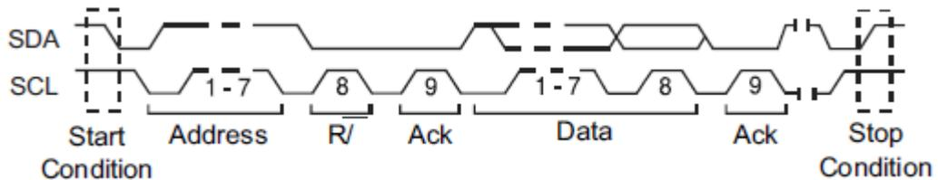
**Restart** — The oscilloscope will be triggered when another “Start” occurs before a “Stop”.
