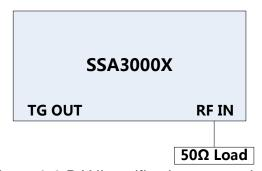
Figure 3-3 DANL verification connections
