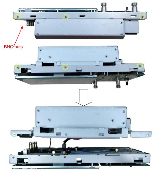
Figure 4-3 Removing the rear metal cover
