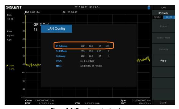
Figure 2-2 IP configuration interface
