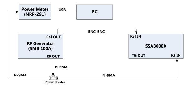
Figure 3-2 Frequency response connections
