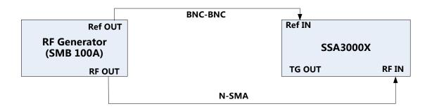
Figure 3-4 Phase noise verification connections
