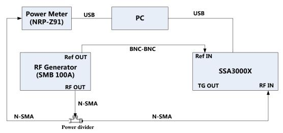
Figure 3-1 Absolute amplitude accuracy connections
