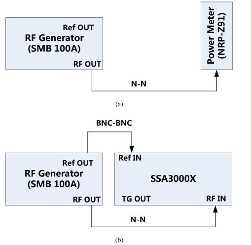
Figure 3-9 connecting test instruments for Input Attenuation Error Test
