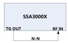
Figure 3-10 Connecting test instruments for TG Output
