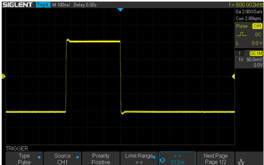
Figure 26 Pulse Trigger
