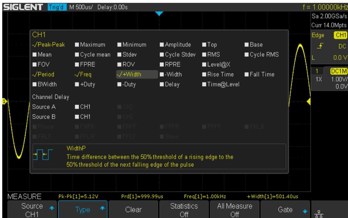
Figure 66 Select the Measurement Parameter
