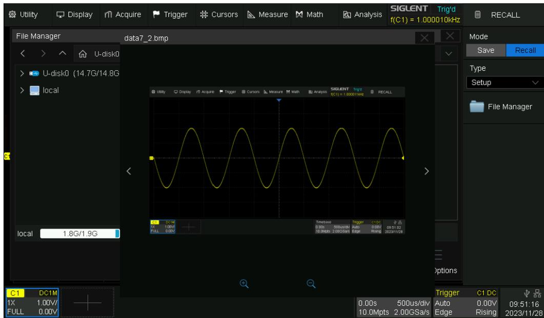
**Recall the setup file "track.xml" stored in path "U-disk0\sds1khd"**
