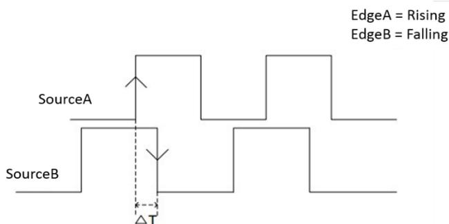
Click the **SourceB Setting** region to set the edge trigger source, threshold, and slope.
