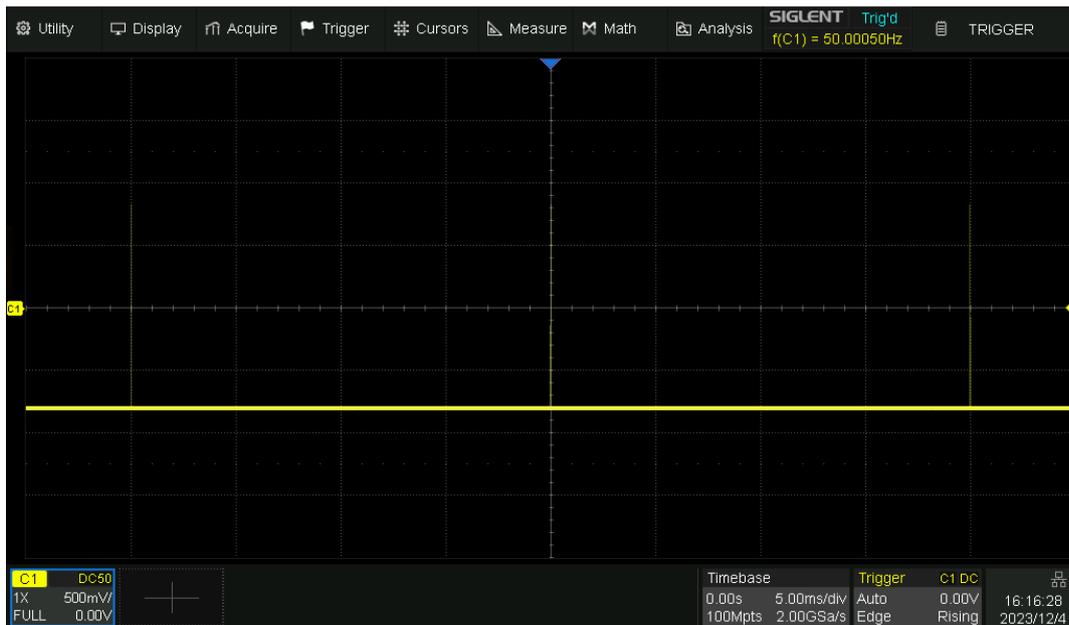
In normal mode, 3 pulses can be obtained on the screen with the sample rate of 2GSa/s at the maximum memory depth.
