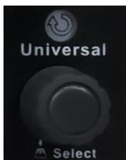
When the parameter setting area is highlighted, the Universal Knob can be used to adjust the parameter. Press the knob to select an option from the list. The default function of the Universal Knob is to adjust the intensity of the waveform traces.
