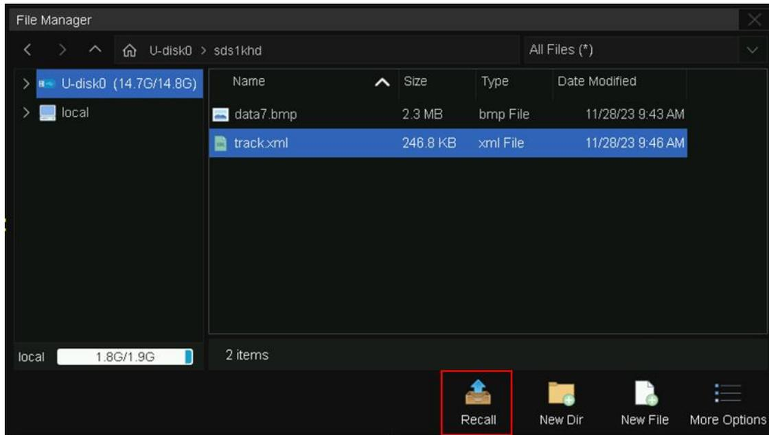
Fourth, touch the Recall icon
