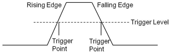
Touch the **Source** area to select trigger source, and touch the **Slope** area to select rising, falling, or alternating.
