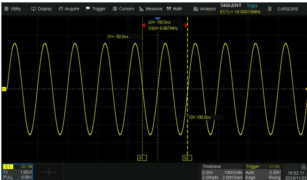
Fixed delay, timebase is changed to 100 ns/div, the value of X cursors (-50 ns, 100 ns) remains fixed. The grid number of X cursors is changed to -0.5div, 1div.
