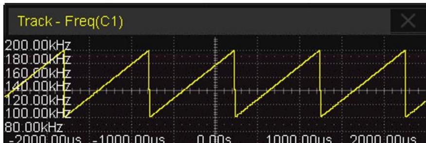
The upper limit of the statistic number in a frame is set in **Statistics Setting** > **AIM Limit**, which means the values exceeding the limit will not be shown in the track plot.
