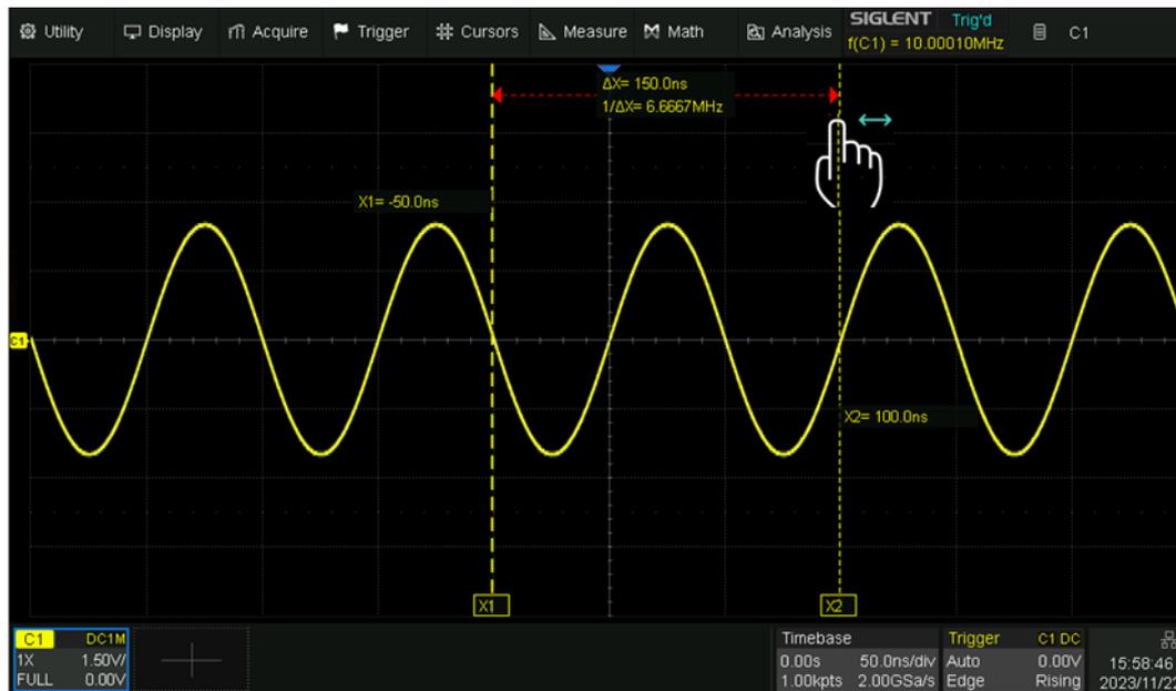
Touch the display area of  $\Delta X$  (or  $\Delta Y$ ) in Following mode and drag it to move the two cursors simultaneously, as shown in the figure below. This is equivalent to the operation on the cursor type X1-X2 or Y1-Y2.
