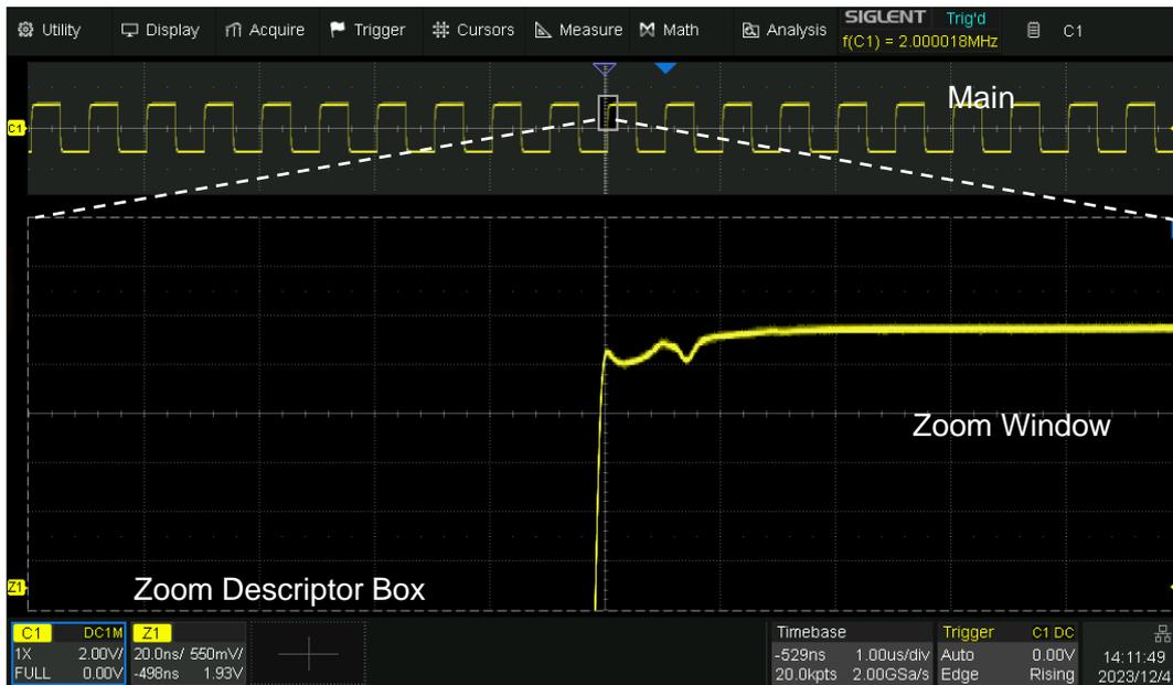
The area not covered by the gray background in the main waveform area is the range to be zoomed in (zoom area). Touch the Zoom Vertical Parameters and Zoom Horizontal Parameters regions shown in the figure above to recall the quick dialogs for setting the vertical and horizontal parameters of the zoom window.
