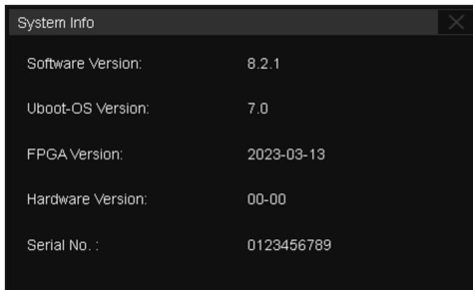
**System Info** – Includes Software Version,Uboot-OS Version, FPGA Version,Serial Number and Hardware Version of the SLA1016 probe.
