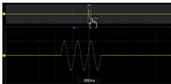
Adjust the horizontal position of the waveform by dragging left and right in the gray area of the main window
