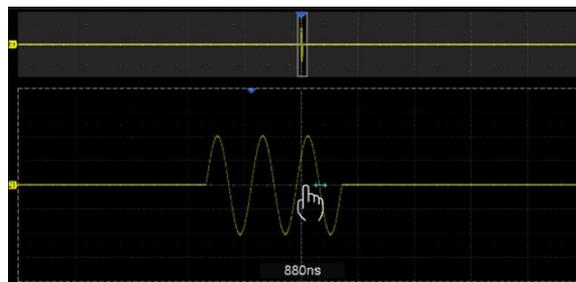
Adjust the horizontal position of the zoom area by dragging left and right in the zoom area of the main window or waveform in the Zoom window
