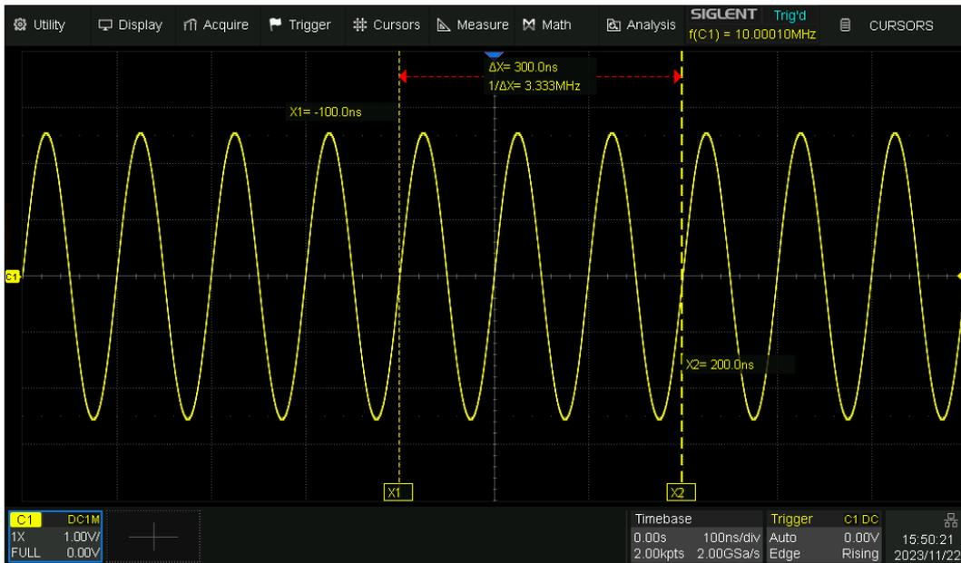
Fixed position, timebase is changed to 100 ns/div, the grid number of X cursors (-1div, 2div) remains fixed. The value of X1 and X2 is changed to -100 ns, 200 ns.
