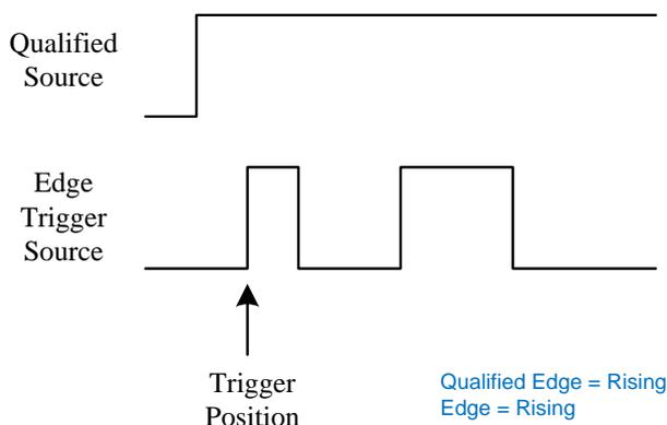
Click the **Qualified Setting** region to set the qualified source and threshold; Click the **Edge Setting** region to set the edge trigger source, threshold, and slope.
