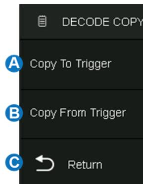
**Note:** The synchronization is not automatic. If the settings at one place change, a copy operation is necessary to re-synchronize.
