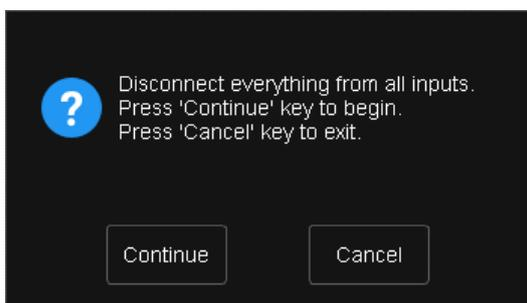
3. The oscilloscope will not respond to any operation until the self-cal is finished. After the self-cal is completed, touch the screen or press any button to exit.
