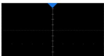
**Trigger Delay Indicator** locates where the waveform triggers on the horizontal axis... When the trigger position is outside the screen, the direction of the triangle points outside the screen as well.
