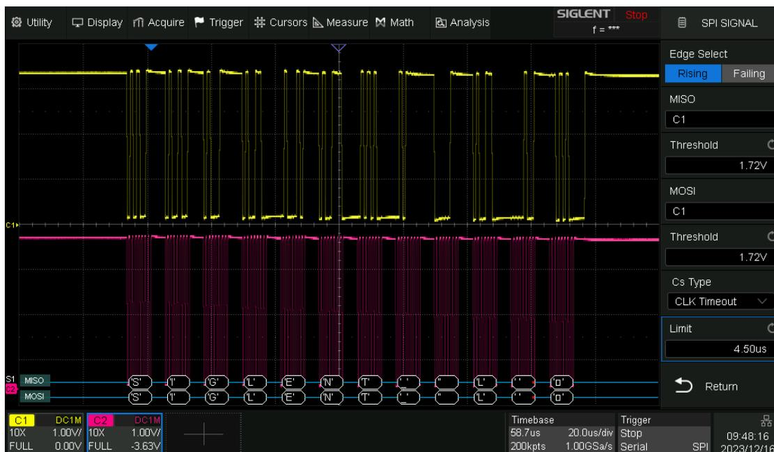
If the data width is set to be greater than 8 bits (such as 16 bits), measure the clock idle time between 8-bit data packets as 5.05 us, and then set the timeout time to a value between 5.05 and 500 us. In this example, it is set to 80 us:
