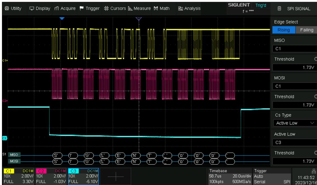
When the CS type is set to CLK Timeout, turn on Cursor, measure the clock idle time between frames as 505 us, and measure the interval between clock pulses as 0.5 us, then set the timeout to a value between 0.5 us and 505 us. In this example it is set to 4.5 us:
