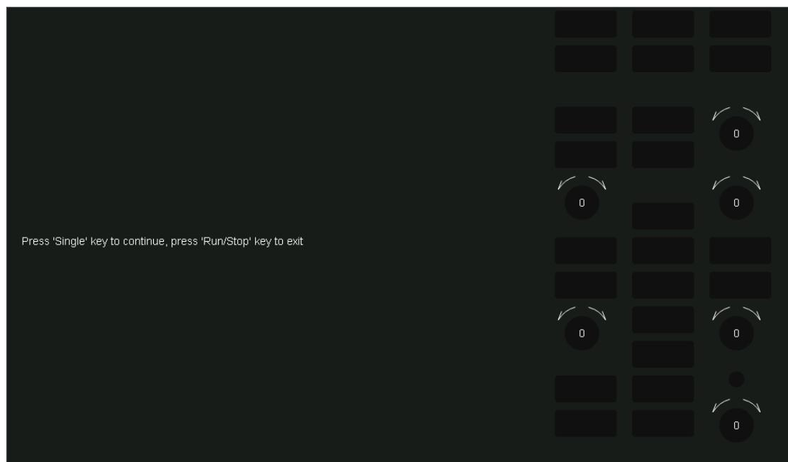
Press the "Single" button and the first LED on the front panel will light. The corresponding position of the key on the screen will also change color. Press the "Single" button to check the next button. Press the "Single" button consecutively until all the backlights are tested. Press the "Run/Stop" button to exit the LED test.
