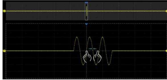
Adjust the horizontal scale of the Zoom window by horizontal pinch and spread in the zoom area of the main window or the Zoom window
