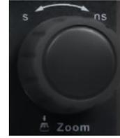
When the Zoom function is on, the waveform area is divided into upper and lower parts. The area of about 1/3 height above is the main window, and the area of about 2/3 height below is the zoom window. Touch a window to activate it. The currently activated window is highlighted by the dashed line.
