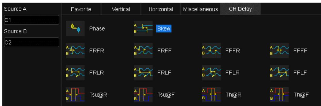
In the parameter selection area, the channel corresponding to **Source A** is specified first, and then the channel corresponding to **Source B**. Finally, the measurement parameter is selected. For example, to activate the skew between C1 and C2, you can follow the following steps:
