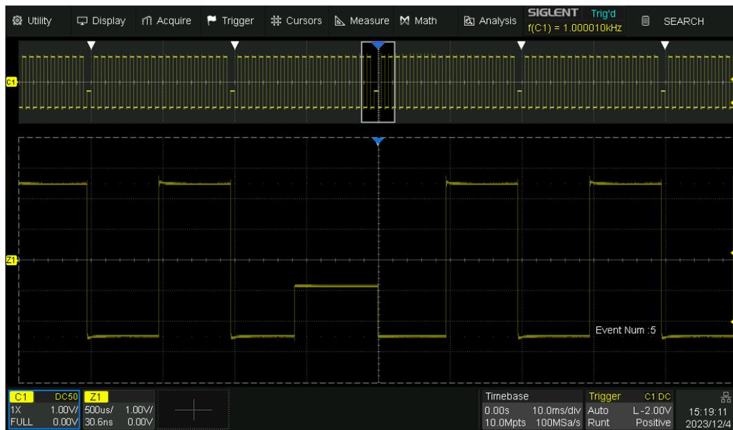
Press the **Run/Stop** button on the front panel to stop the acquisition, and then follow the steps **Navigate** > **Type** to select “Search Event”. The following figure shows the first dwarf pulse. In this example, the list is enabled and the time labels of a partial event are shown in the list.
