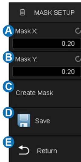
Set the values for **Mask X** and **Mask Y** (in divisions of display graticule), and then perform **Create Mask** to generate the mask. The horizontal and vertical adjustment range is 0.04~4.00 div.
