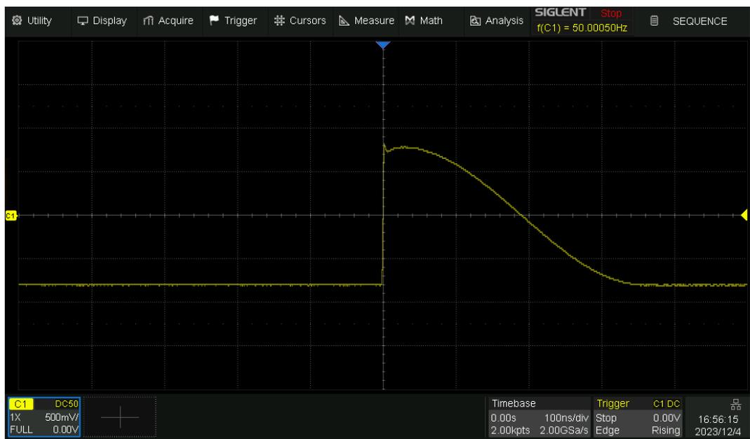
In the example, 45976 pulses can be obtained with the sample rate of 2 GSa/s at the maximum memory depth.
