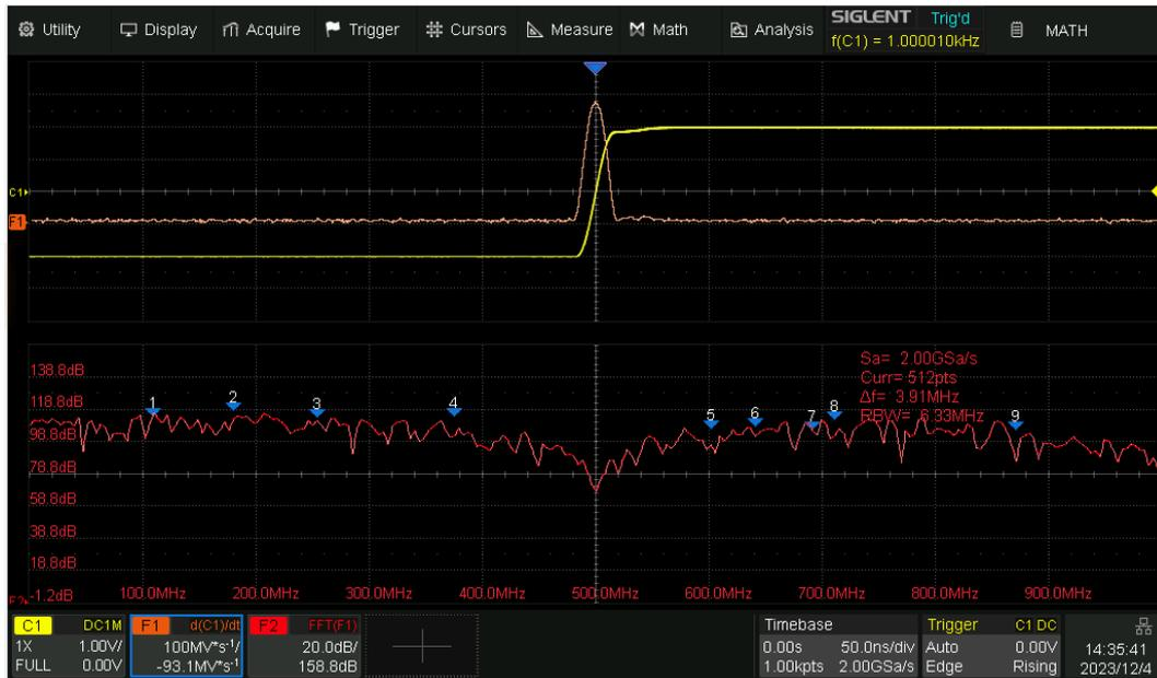
In this example,  $F1 = d(C1)/dt$  and  $F2 = \text{FFT}(d(C1)/dt)$  are equivalent to  $F2 = \text{FFT}(F1)$ , which is equivalent to performing FFT analysis on the differential operation results of C1 waveform.
