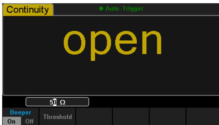
Diagram 2- 36 Set Up the Short-circuit Resistance
