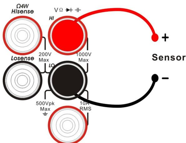
Diagram 3- 13 Sketch map for connecting the sensor
