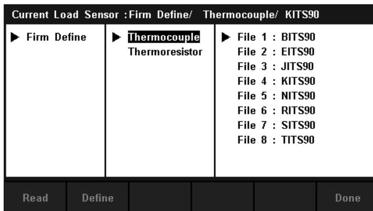
Diagram 3- 14 Select the Type of Thermocouple
