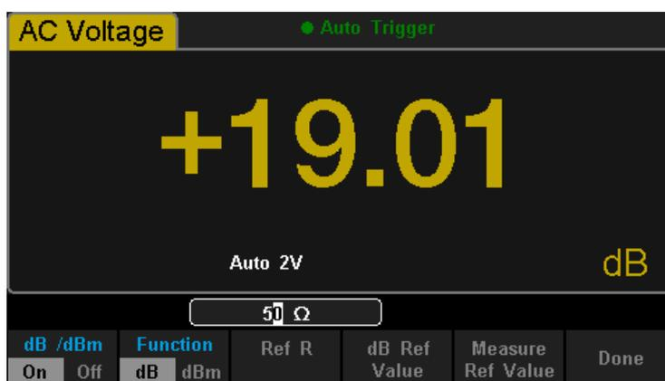
Diagram 3- 8 Set the Parameters of dB
