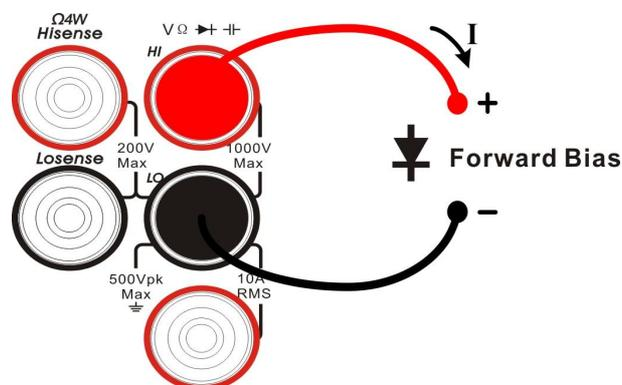
Diagram 2- 26 Sketch Map for testing Diode
