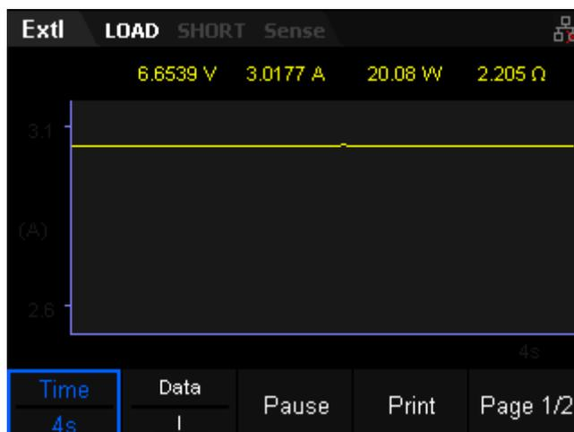
Figure 3-13 Waveform display interface of ExtI mode
