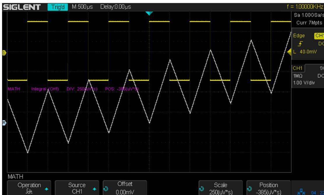
Figure 48 Integral with Offset
