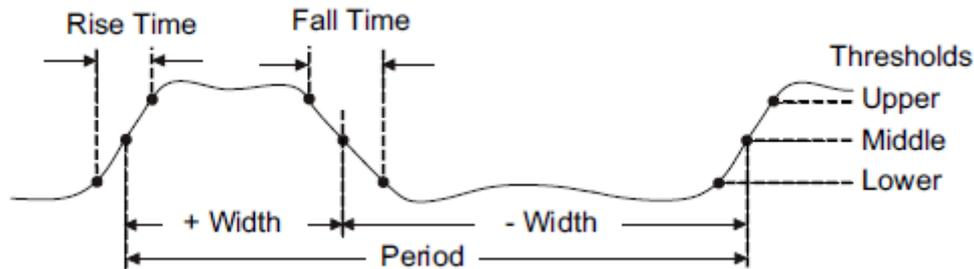
Figure 54 Time Measurements
