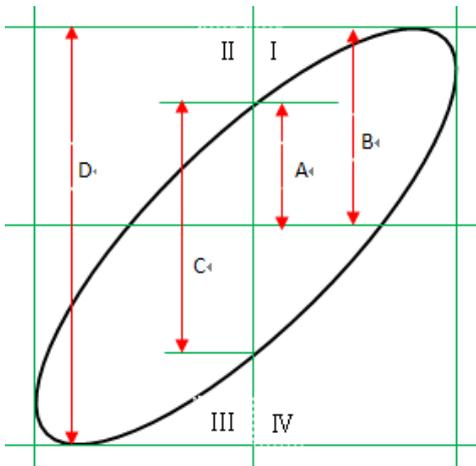
According to  $\sin\theta=A/B$  or  $C/D$  (wherein,  $\theta$  is the phase deviation angle between the two channels and the definitions of A, B, C and D are as shown in the figure above), the phase deviation angle is obtained, that is:  $\theta=\pm\arcsin(A/B)$  or  $\pm\arcsin(C/D)$
