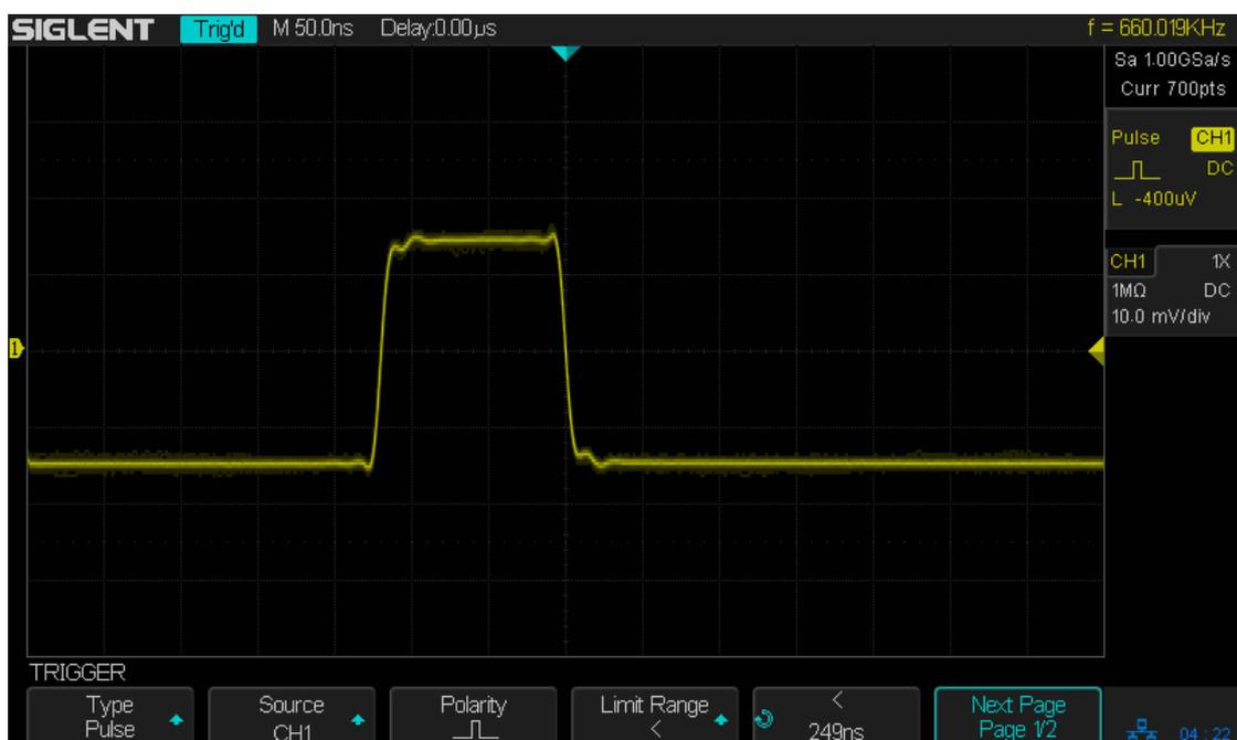
Figure 25 Pulse Trigger
