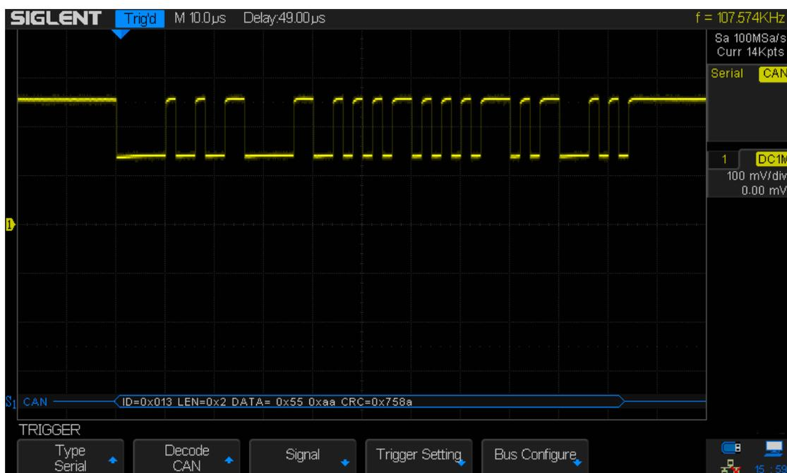
Figure 56 CAN Trigger
