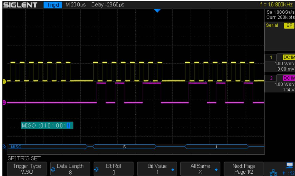
Figure 48 SPI Trigger
