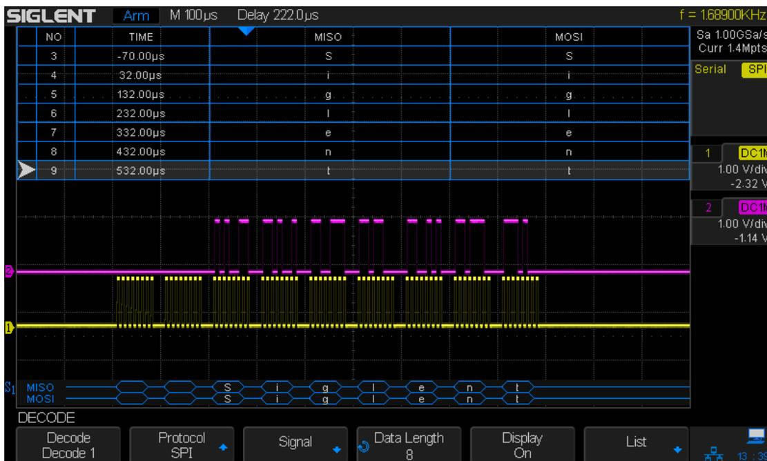
Figure 49 SPI Decode
