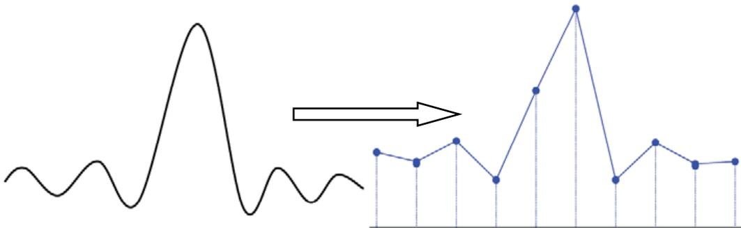
2. **Waveform Confusion:** when the sample rate is lower than twice the actual signal frequency (Nyquist Frequency), the frequency of the waveform rebuilt from the sample data is lower than the actual signal frequency. The most common aliasing is the jitter on fast edge.
