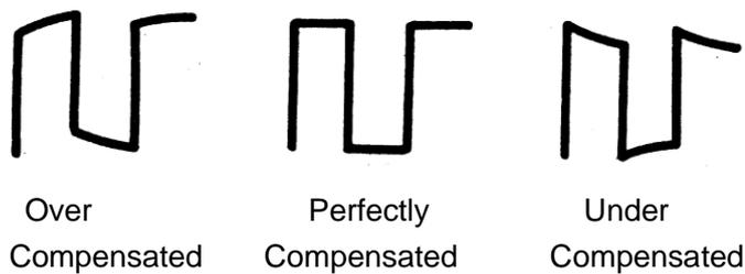
4. Use a nonmetallic driver to adjust the low-frequency compensation adjustment hole on the probe until the waveform displayed is as the “Perfectly compensated” in the figure above.
