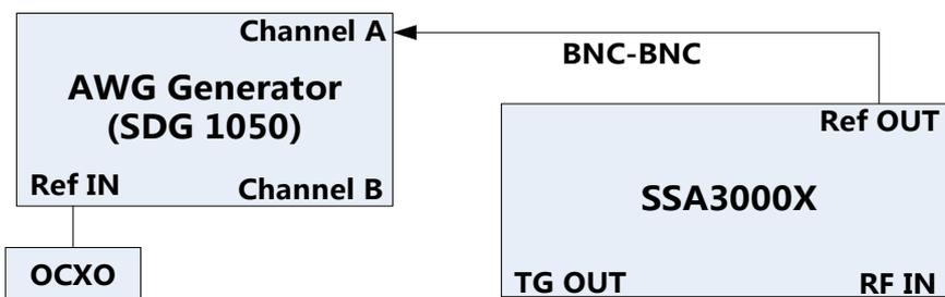
Figure 3-6 Connecting test instruments for frequency accuracy
