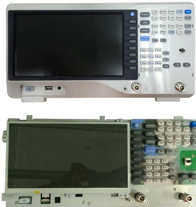
Figure 4-2 Removing the front panel
