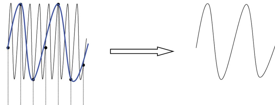
3. **Waveform Leakage:** when the sample rate is too low, the waveform rebuilt from the sample data does not reflect all the actual signal information.
