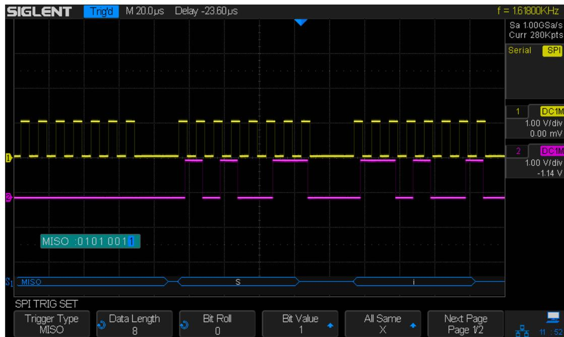
Figure 45: SPI Trigger
