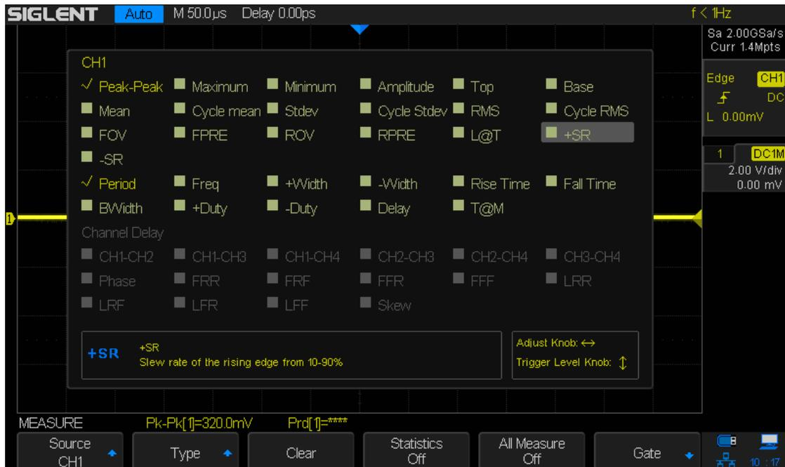
Figure 78: Select the Measurement Parameter
