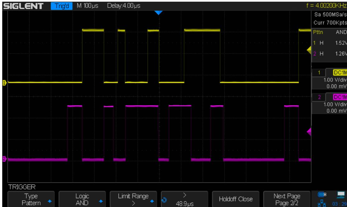
Figure 34: Pattern Trigger
