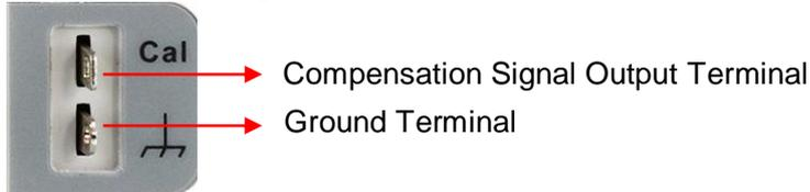
3. Use the probe to connect the input terminal of CH1 of the oscilloscope and the “Compensation Signal Output Terminal” of the probe.
