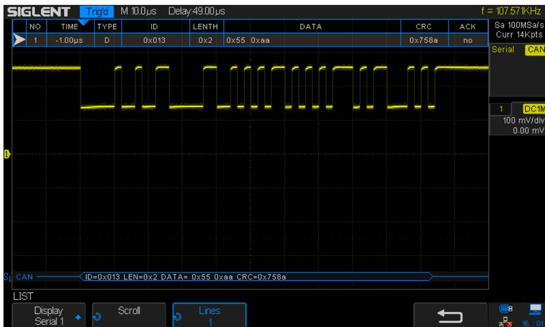
Figure 54: CAN Decode
