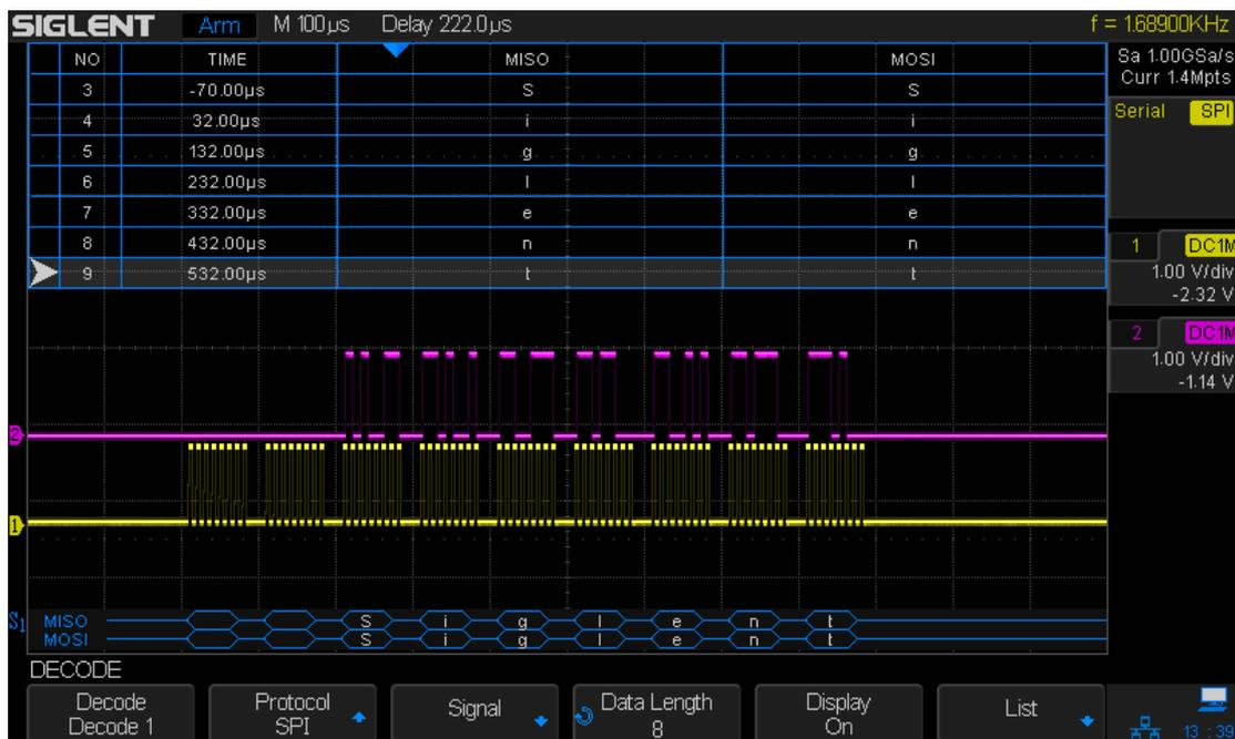
Figure 46: SPI Decode
