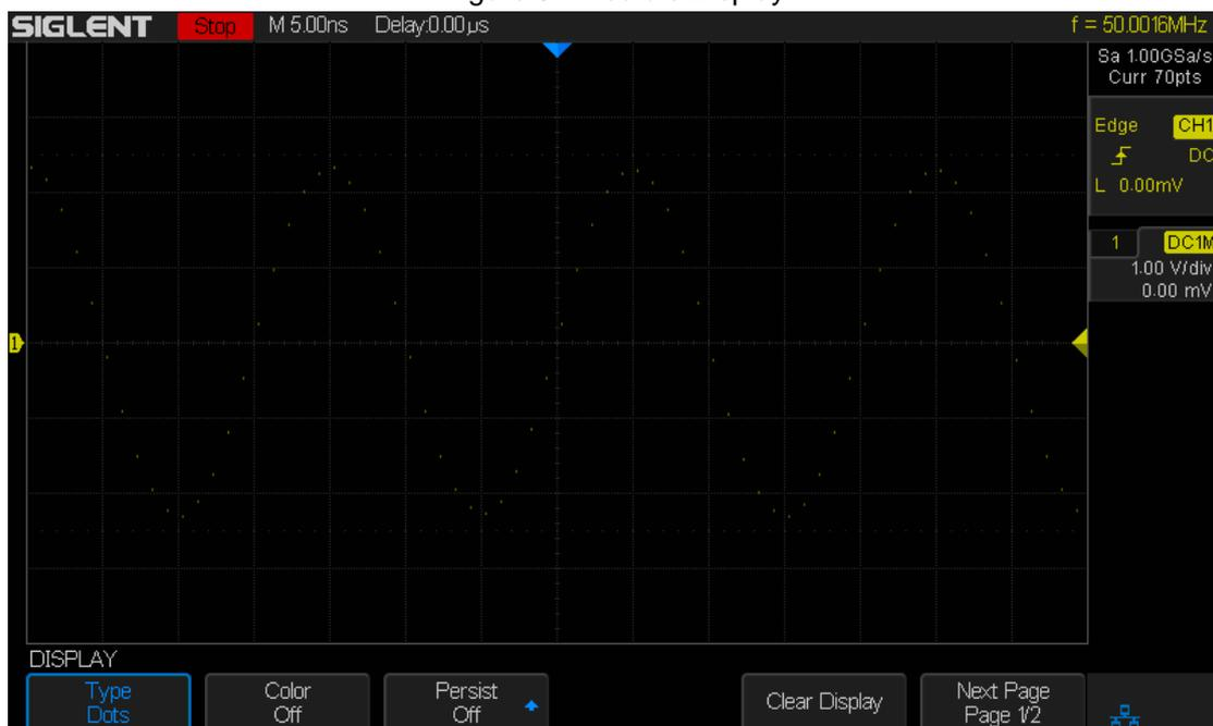
Figure 82: Dots Display
