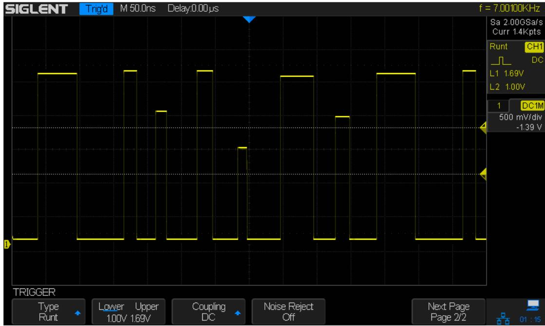
Figure 33: Runt Trigger
