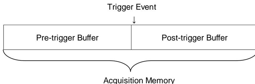
The trigger setting should be based on the type of signal characteristics of the input signal, thus a certain amount of knowledge about the signal-under-test is helpful in order to quickly capture the desired waveform.
