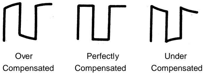
4. Use a nonmetallic flat-head screwdriver to adjust the low-frequency compensation adjustment hole on the probe until the waveform matches the “Perfectly Compensated” waveform above.
