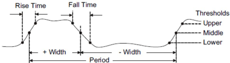
Figure 77: Time Measurements
