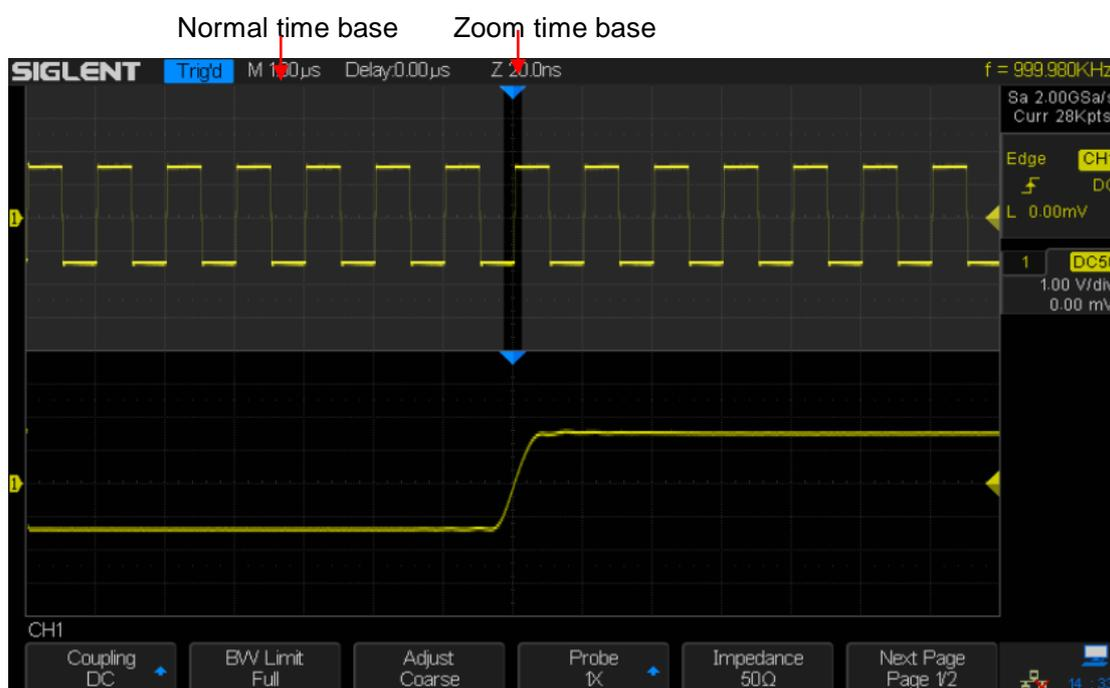
The area of the normal display that is expanded is outlined with a box and the rest of the normal display is ghosted. The box shows the portion of the normal sweep that is expanded in the lower half.
