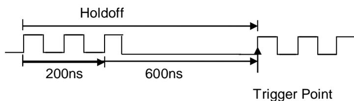
The correct holdoff setting is typically slightly less than one repetition of the waveform. Set the holdoff to this time to generate a unique trigger point for a repetitive waveform. Only edge trigger and serial triggers have the holdoff option. The holdoff time of SDS2000X is adjustable from 100ns to 1.5s.
