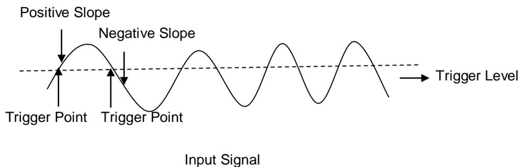
The trigger level can be adjusted for a selected analog channel by turning the **Trigger Level Knob**.
