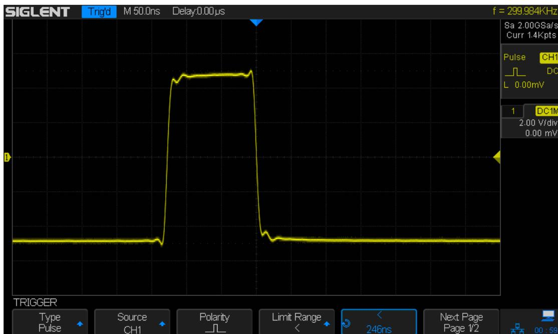
Figure 26: Pulse Trigger
