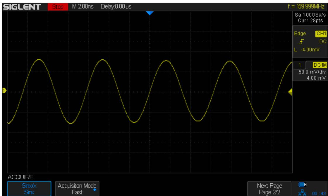
Figure 13: Sinx/x Interpolation
