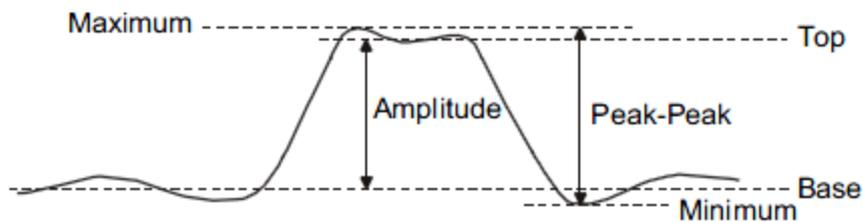
Figure 74: Voltage Measurements
